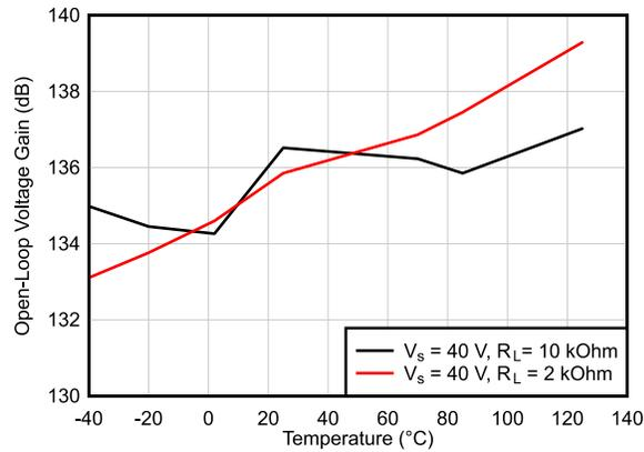
Figure 5-21. Open-Loop Voltage Gain vs Temperature (dB)
