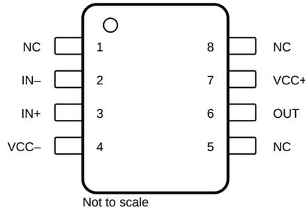
**Figure 4-3. TL081x: D Package, 8-Pin SOIC,
