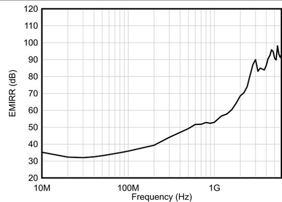
Figure 5-36. EMIRR (Electromagnetic Interference Rejection Ratio) vs Frequency
