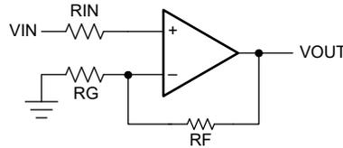
**Figure 8-4. Operational Amplifier Schematic for Non-inverting Configuration**
