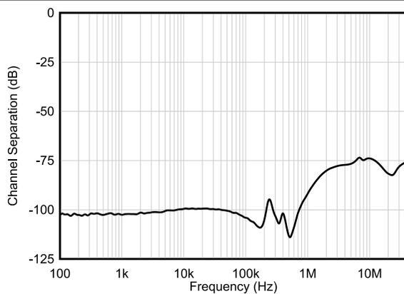
Figure 5-35. Channel Separation vs Frequency
