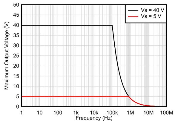
Figure 5-34. Maximum Output Voltage vs Frequency
