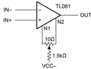
**Figure 6-4. Test Figure 4 (for SO Package Only)**
