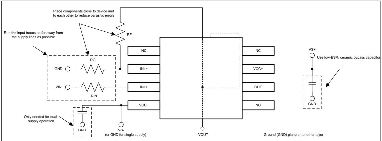
**Figure 8-3. Operational Amplifier Board Layout for Non-inverting Configuration**
