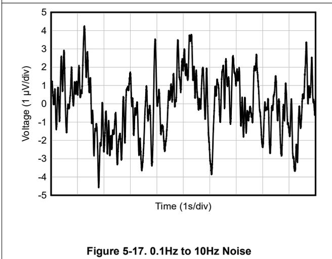
Figure 5-17. 0.1Hz to 10Hz Noise
