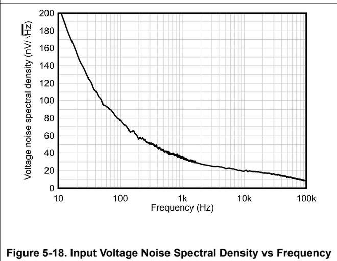
Figure 5-18. Input Voltage Noise Spectral Density vs Frequency
