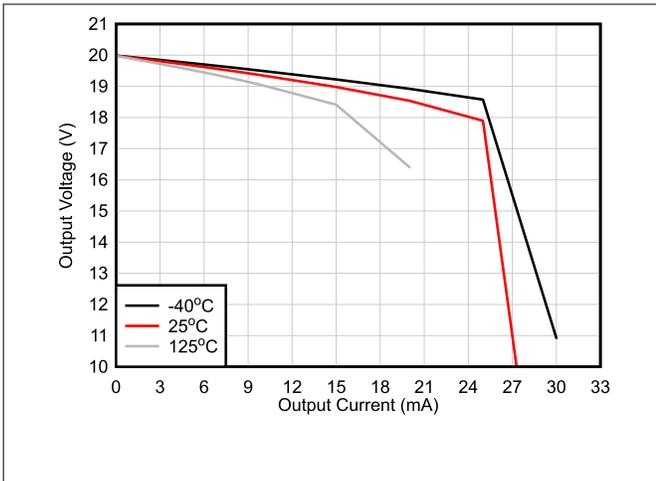
Figure 5-13. Output Voltage Swing vs Output Current (Sourcing)
