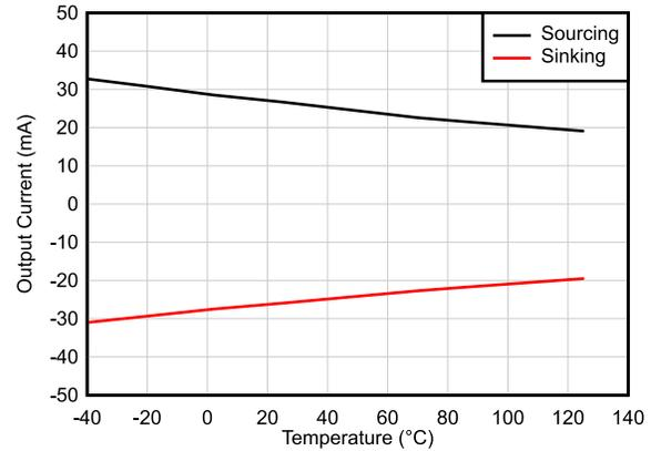
Figure 5-22. Short-Circuit Current vs Temperature
