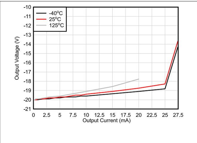
Figure 5-14. Output Voltage Swing vs Output Current (Sinking)
