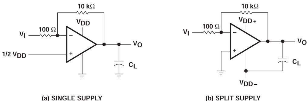
Figure 6-3. Gain-of-100 Inverting Amplifier
