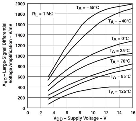
**Figure 5-15. Large-signal Differential Voltage Amplification vs Supply Voltage**
