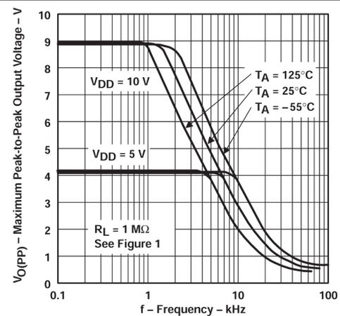
Figure 5-24. Maximum Peak-to-peak Output Voltage vs Frequency
