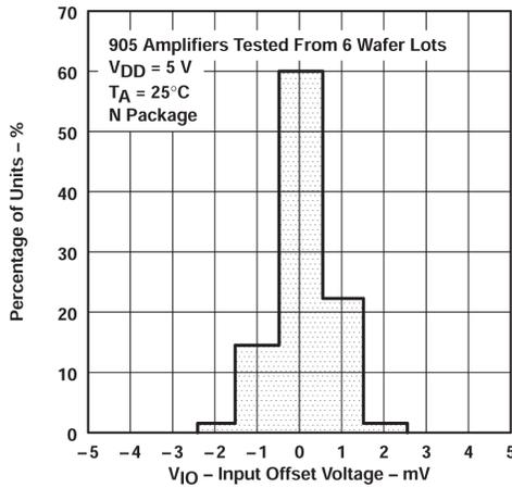
**Figure 5-1. Distribution of TLC27L4 Input Offset Voltage**
