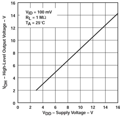
Figure 5-7. High-level Output Voltage vs Supply Voltage
