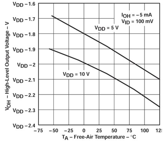
Figure 5-8. High-level Output Voltage vs Free-air Temperature
