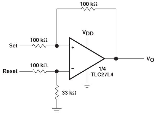
Figure 7-10. Set/Reset Flip-Flop,  $V_{DD} = 5V$  to  $16V$
