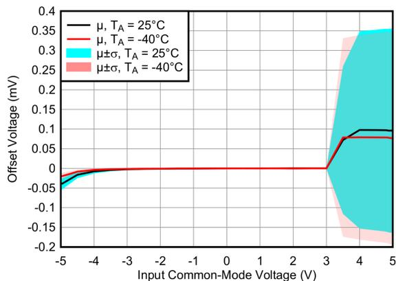
**Figure 7-3. Offset Voltage vs Input Common-Mode Voltage**
