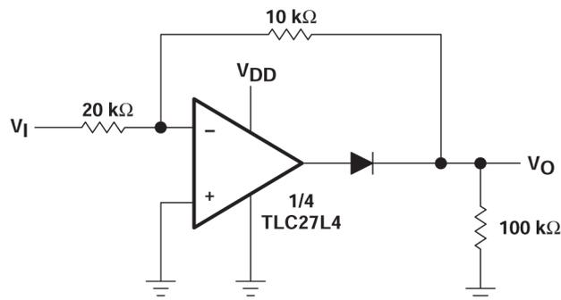
Figure 7-12. Full-Wave Rectifier,  $V_{DD} = 5V$  to  $16V$
