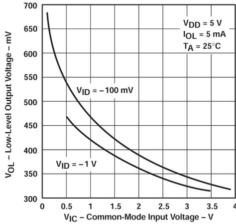
Figure 5-9. Low-level Output Voltage vs Common-mode Input Voltage
