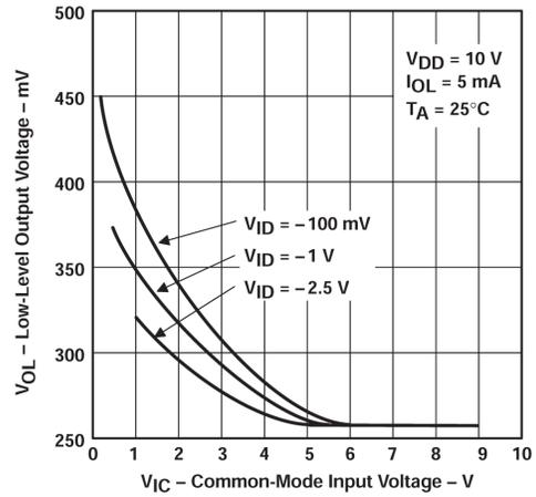
Figure 5-10. Low-level Output Voltage vs Common-mode Input Voltage
