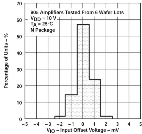
**Figure 5-2. Distribution of TLC27L4 Input Offset Voltage**
