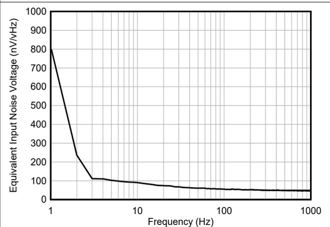
**Figure 5-30. Equivalent Input Noise Voltage vs Frequency**
