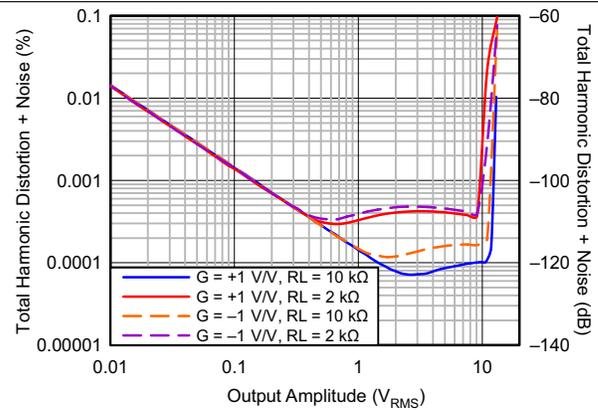
$f = 1\text{ kHz}$ ,  $BW = 80\text{ kHz}$
