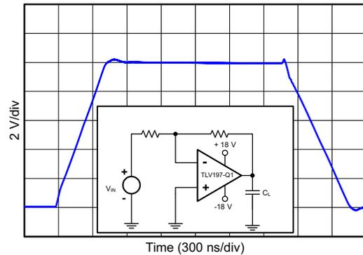
$R_L = 1\text{ k}\Omega$ ,  $C_L = 10\text{ pF}$ ,  $G = -1$
