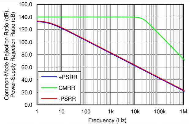
Figure 10. CMRR and PSRR vs Frequency
