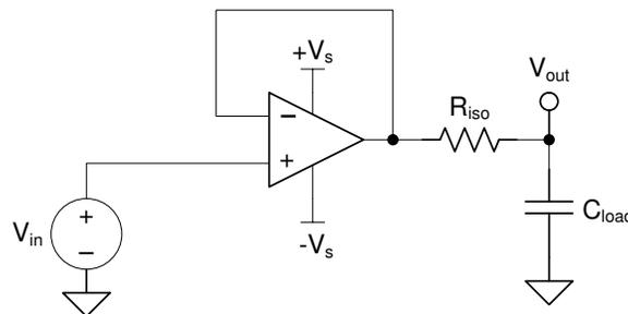
**Figure 38. Extending Capacitive Load Drive With the TLVx197-Q1**
