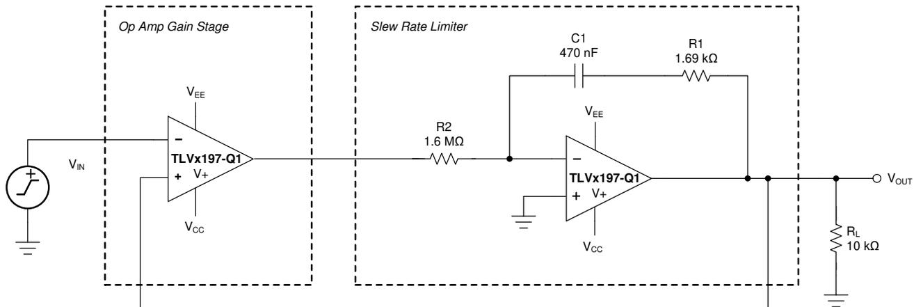
**Figure 43. Slew-Rate Limiter Uses One Op Amp**
