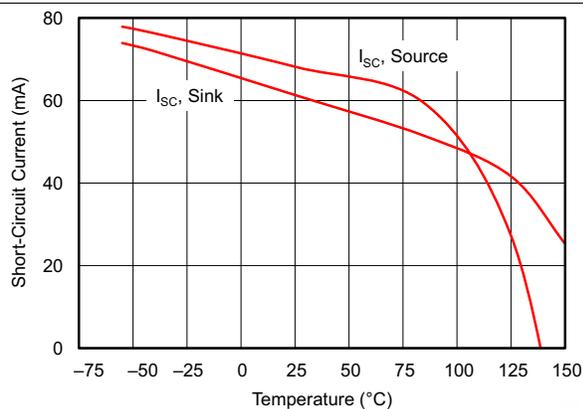
Figure 29. Short-Circuit Current vs Temperature
