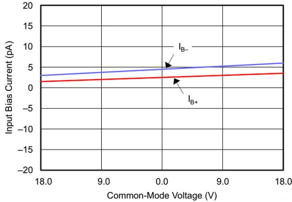
Figure 7. Input Bias Current vs Common-Mode Voltage
