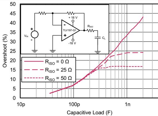
$R_I = 1\text{ k}\Omega$ ,  $R_F = 1\text{ k}\Omega$ ,  $G = -1$
