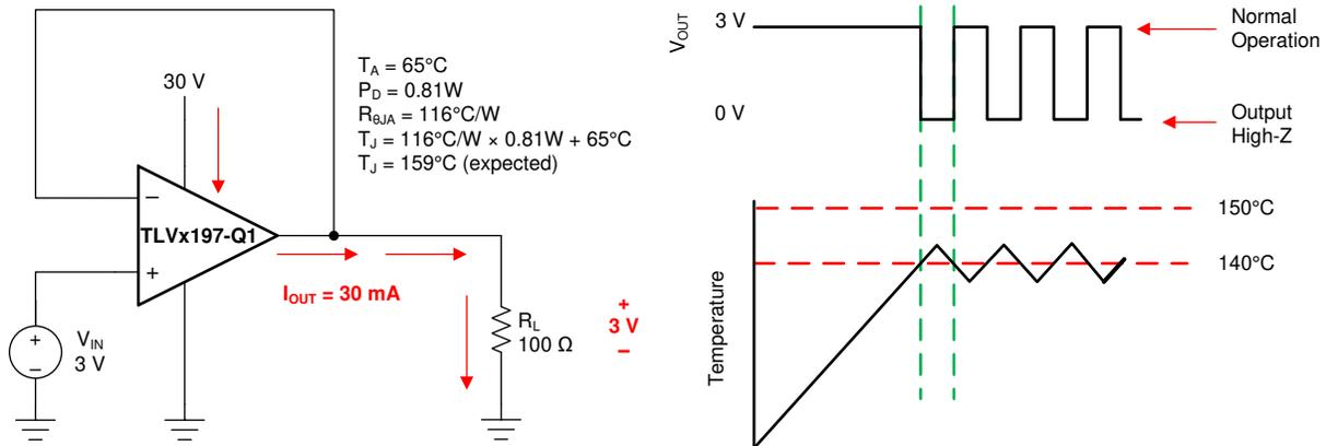
Figure 37. Thermal Protection
