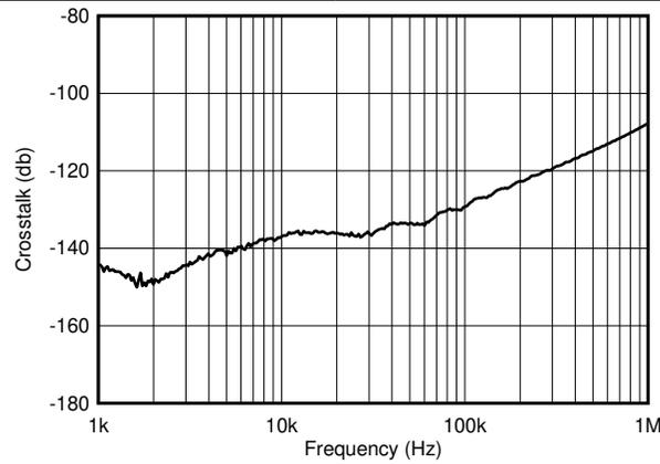
Figure 33. Crosstalk vs Frequency
