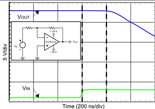
$R_I = 1\text{ k}\Omega$ ,  $R_F = 10\text{ k}\Omega$ ,  $G = -10$
