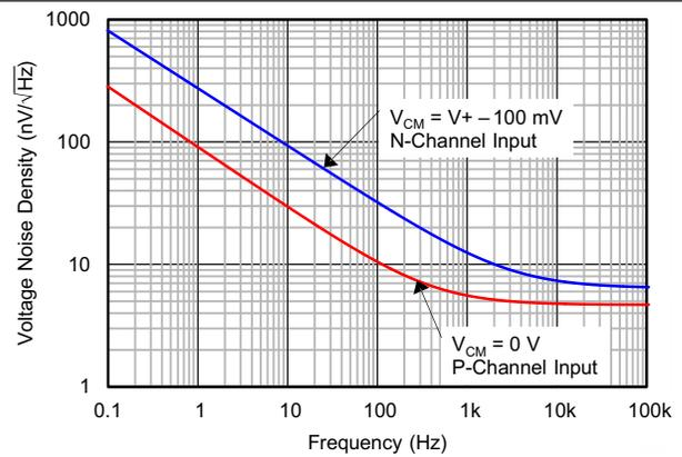
Figure 14. Input Voltage Noise Spectral Density vs Frequency
