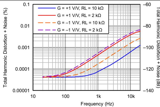
$V_{OUT} = 3.5 V_{RMS}$ ,  $BW = 80\text{ kHz}$
