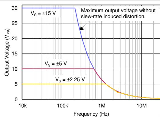
Figure 30. Maximum Output Voltage vs Frequency
