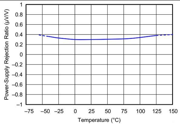
Figure 12. PSRR vs Temperature
