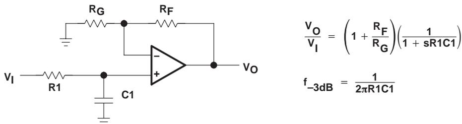
Figure 51. Single-Pole Low-Pass Filter
