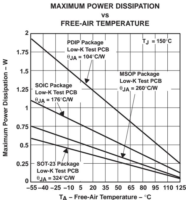
NOTE A: Results are with no air flow and using JEDEC Standard Low-K test PCB.
