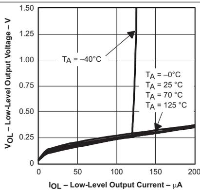
Figure 17. Low-Level Output Current vs Low-Level Output Current
