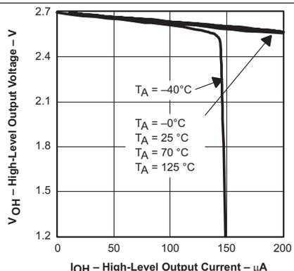
Figure 12. High-Level Output Voltage vs High-Level Output Current
