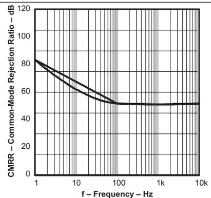
Figure 11. Common-Mode Rejection Ratio vs Frequency
