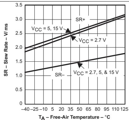
Figure 24. Slew Rate vs Free-Air Temperature
