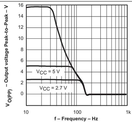
Figure 18. Output Voltage Peak-to-Peak vs Frequency
