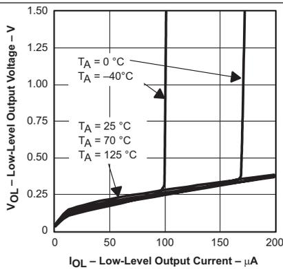
Figure 15. Low-Level Output Voltage vs Low-Level Output Current
