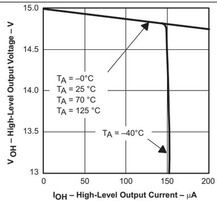
Figure 16. High-Level Output Voltage vs High-Level Output Current
