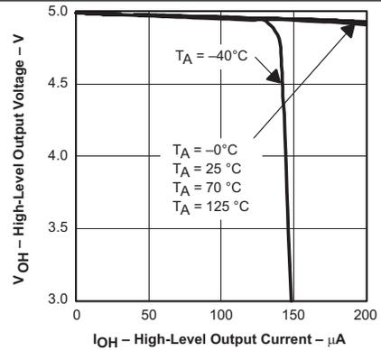
Figure 14. High-Level Output Voltage vs High-Level Output Current
