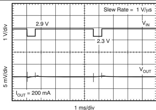
Figure 17. TLV70018 Line Transient Response
