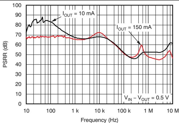
Figure 11. TLV70018 Power-Supply Ripple Rejection vs Frequency
