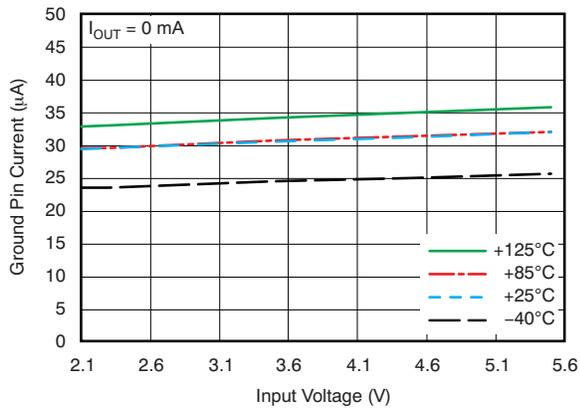
Figure 7. TLV70018 Ground Pin Current vs Input Voltage
