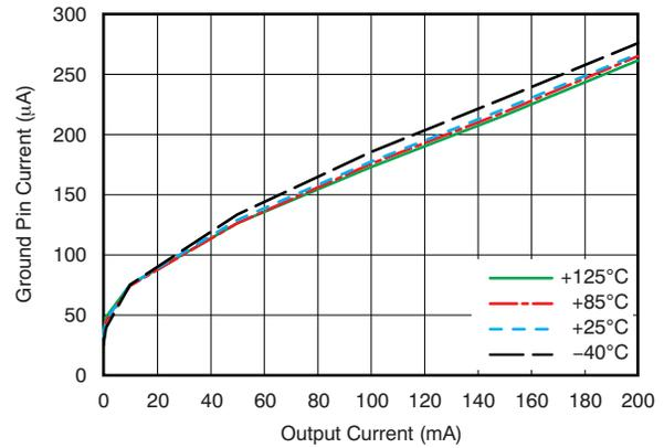
Figure 8. TLV70018 Ground Pin Current vs Load
