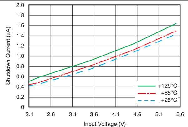
Figure 10. TLV70018 Shutdown Current vs Input Voltage
