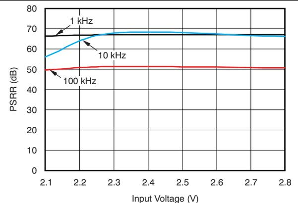
Figure 12. TLV70018 Power-Supply Ripple Rejection vs Input Voltage
