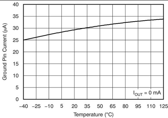
Figure 9. TLV70018 Ground Pin Current vs Temperature
