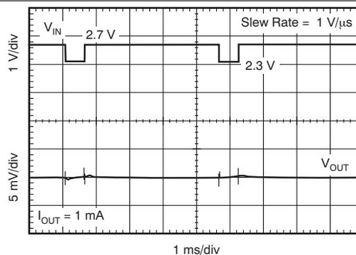
Figure 18. TLV70018 Line Transient Response
