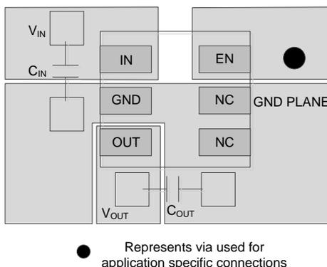
Figure 25. Layout Example for the DSE Package
