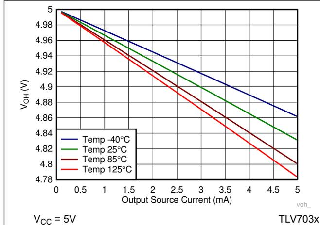
Figure 5-19. Output Voltage High vs Output Source Current
