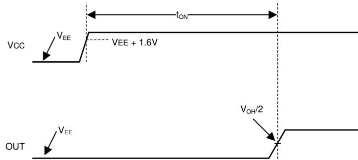
**Figure 5-1. Start-Up Time Timing Diagram (IN+ > IN-)**
