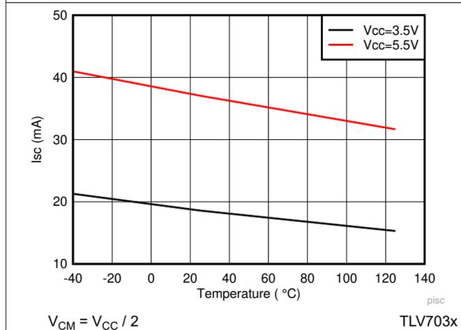
**Figure 5-23. Output Short-Circuit (Source) Current vs Temperature**
