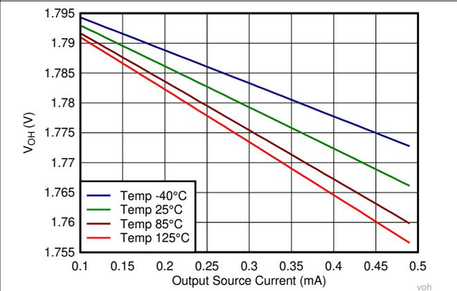
Figure 5-18. Output Voltage High vs Output Source Current
