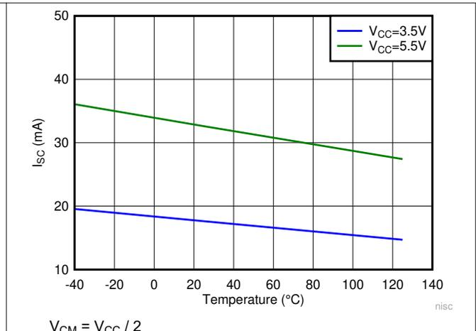
**Figure 5-22. Output Short-Circuit (Sink) Current vs Temperature**
