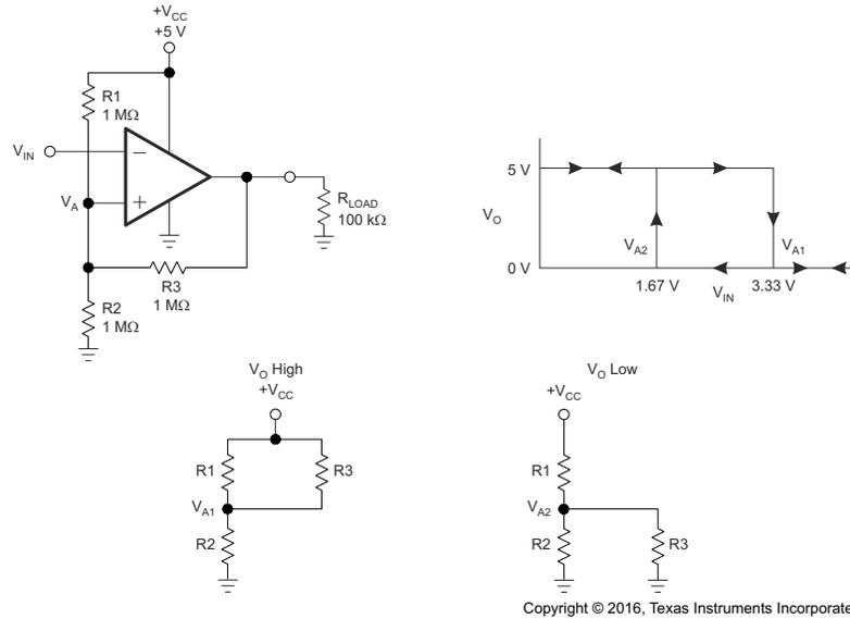
Figure 7-1. TLV703x in an Inverting Configuration With Hysteresis
