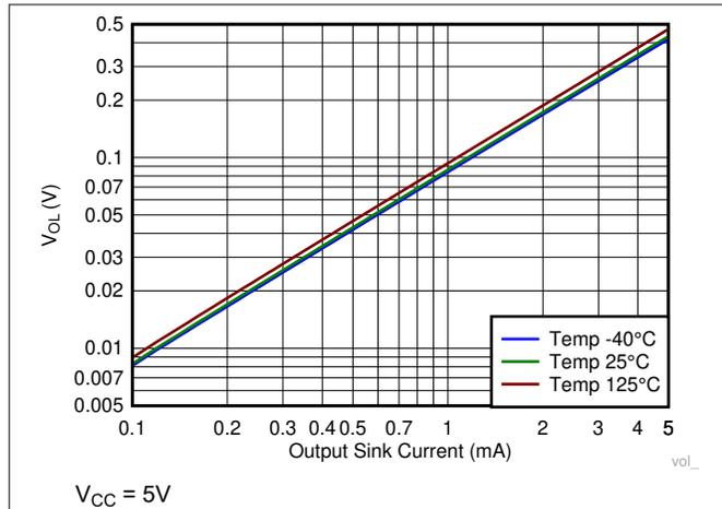
**Figure 5-21. Output Voltage Low vs Output Sink Current**
