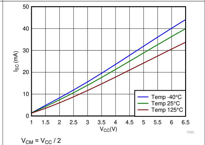
**Figure 5-24. Output Short Circuit (Sink) vs  $V_{CC}$**
