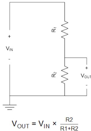
**Figure 7-11. Voltage Divider Equation**
