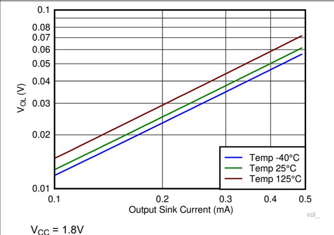
Figure 5-20. Output Voltage Low vs Output Sink Current
