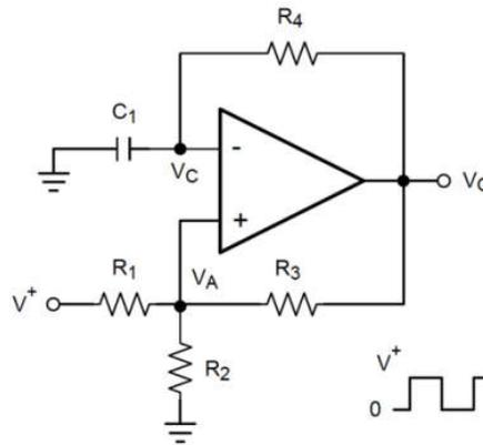
**Figure 7-7. Square-Wave Oscillator**
