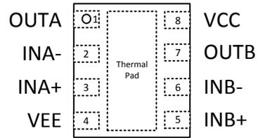
A. Connect thermal pad directly to V– pad.
