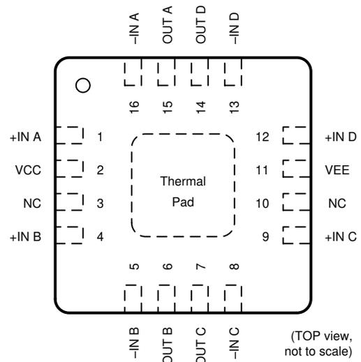
A. Connect thermal pad to V-.
