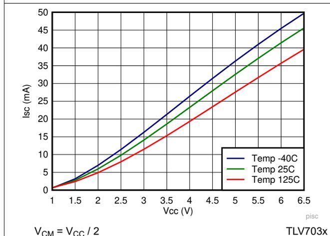
**Figure 5-25. Output Short Circuit (Source) vs  $V_{CC}$**
