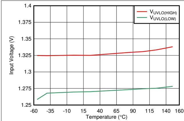
Figure 5-13. UVLO Rising and Falling Threshold vs Temperature
