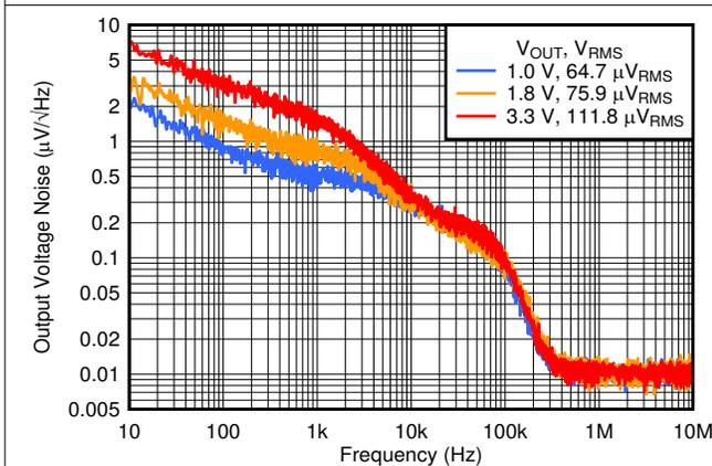
Figure 5-17. Output Noise vs Frequency and  $V_{OUT}$
