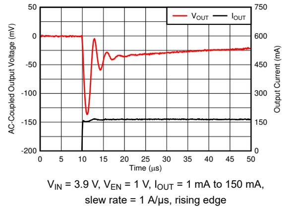
Figure 5-22. Load Transient
