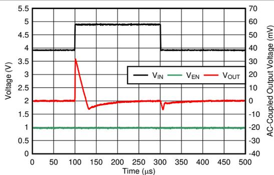
Figure 7-6. VIN Line Transient,  $I_{OUT} = 1$  mA
