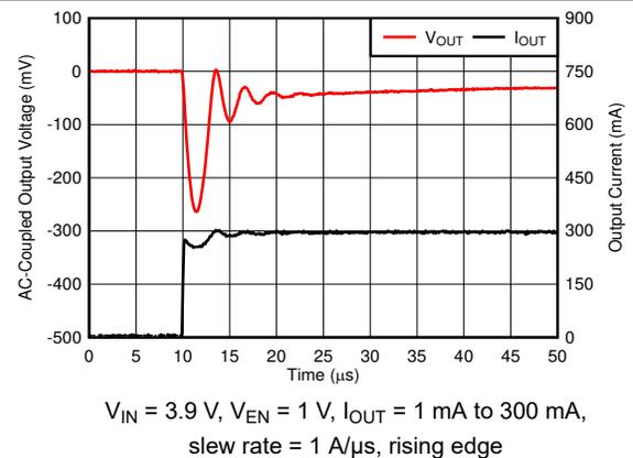
Figure 5-24. Load Transient
