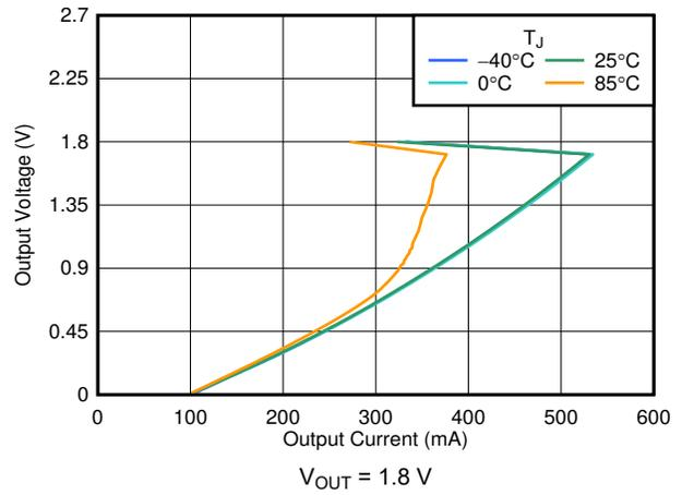
Figure 5-8. Foldback Current Limit vs  $I_{OUT}$
