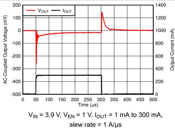
Figure 5-23. Load Transient
