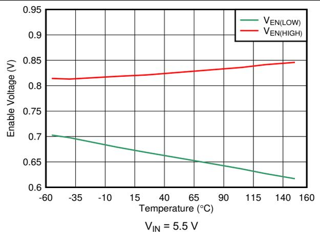
Figure 5-12. EN High and Low Threshold vs Temperature
