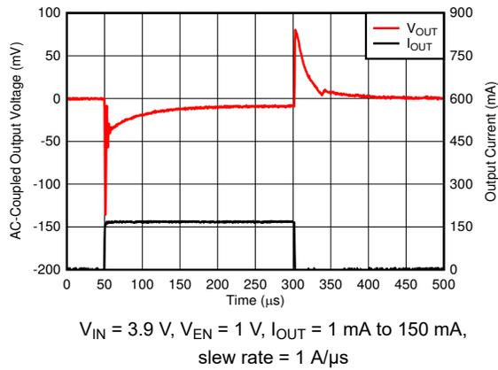
Figure 5-21. Load Transient
