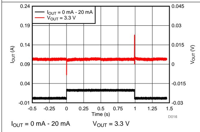
Figure 15. Load Transient
