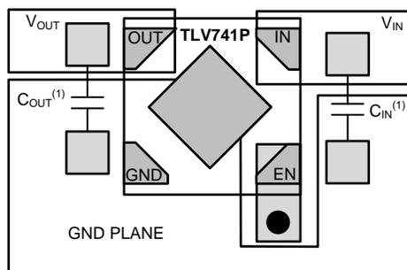
● Represents via used for application-specific connections
