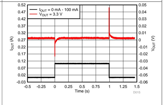
Figure 16. Load Transient
