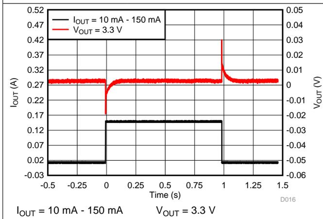
Figure 17. Load Transient
