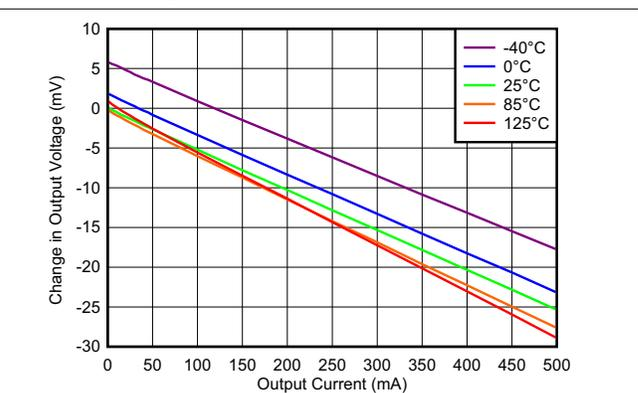
Figure 5-12. Load Regulation vs  $I_{OUT}$
