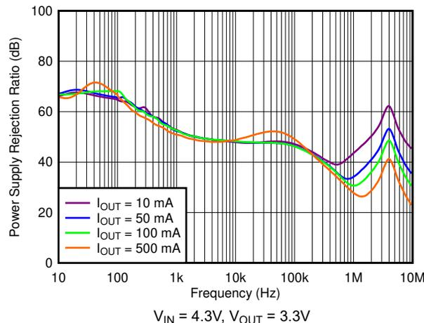
**Figure 7-5. PSRR vs Frequency (4.3V to 3.3V)**
