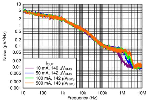
$V_{OUT} = 3.3\text{V}$ ,  $I_{OUT} = 500\text{mA}$ ,  $C_{OUT} = 1\mu\text{F}$ ,  $V_{RMS} \text{ BW} = 10\text{Hz to } 100\text{kHz}$
