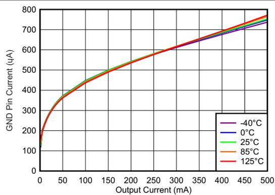
Figure 5-17.  $I_{GND}$  vs  $I_{OUT}$
