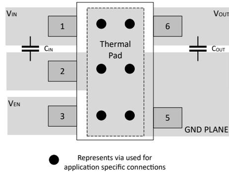
**Figure 7-9. Layout Example for the DYD Package**
