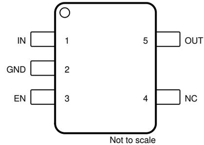
Figure 4-2. DBV Package, 5-Pin SOT-23 (Top View)
