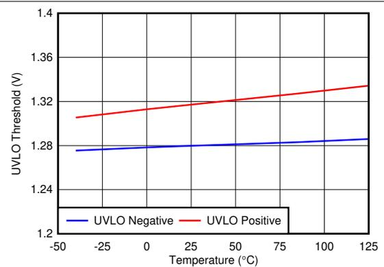
Figure 5-24. UVLO Threshold vs Temperature
