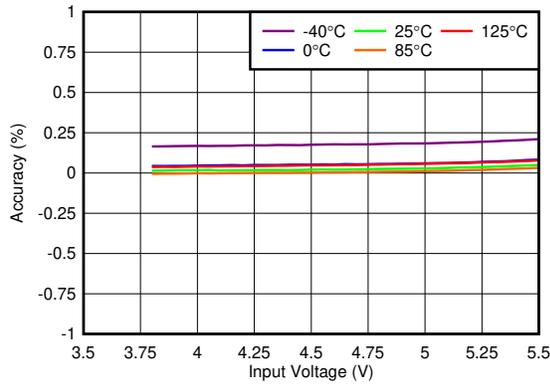
Figure 5-15. 3.3V Regulation vs  $V_{IN}$  (Line Regulation)
