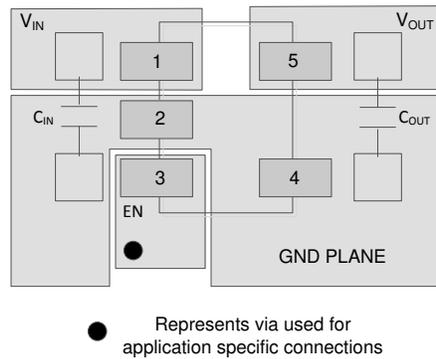
**Figure 7-7. Layout Example for the DBV Package**
