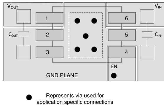
**Figure 7-8. Layout Example for the DRV Package**
