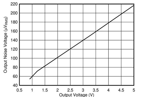
$I_{OUT} = 500\text{mA}$ ,  $C_{OUT} = 1\mu\text{F}$ ,  $V_{RMS} \text{ BW} = 10\text{Hz to } 100\text{kHz}$
