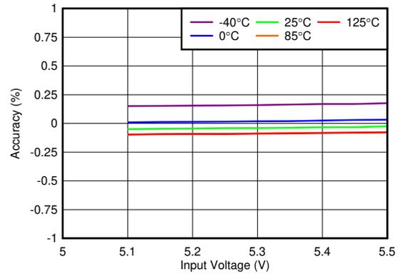
Figure 5-16. 5.0V Accuracy vs  $V_{IN}$  (Line Regulation)
