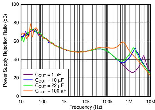
$V_{IN} = 4.3\text{V}$ ,  $V_{OUT} = 3.3\text{V}$ ,  $I_{OUT} = 500\text{mA}$
