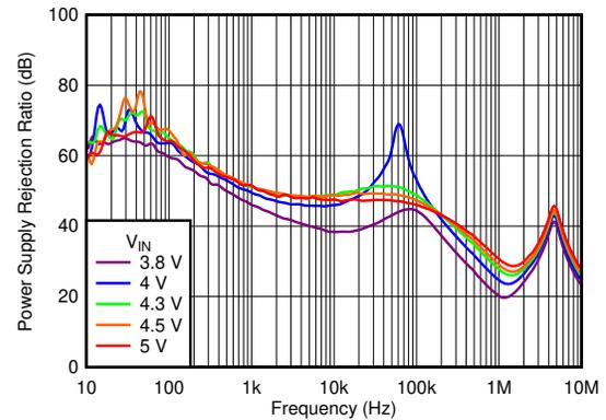
$V_{OUT} = 3.3\text{V}$ ,  $C_{OUT} = 1\mu\text{F}$ ,  $I_{OUT} = 500\text{mA}$
