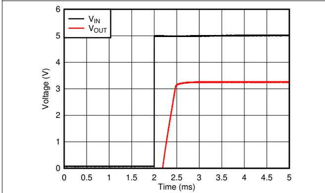
Figure 5-9.  $V_{IN} = V_{EN}$  Power-Up
