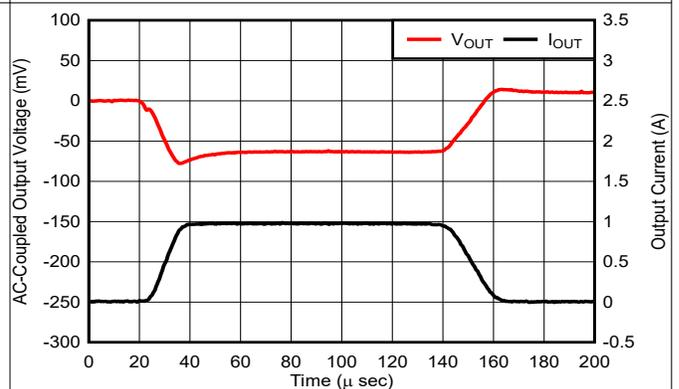
$V_{OUT} = 1.8\text{V}$ ,  $V_{IN} = V_{OUT(nom)} + 1.0\text{V}$ ,  $I_{OUT} = 0\text{mA}$  to  $1\text{A}$  to  $0\text{mA}$ ,
