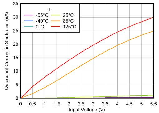
$V_{EN} = 0\text{V}$ ,  $C_{IN} = 0\mu\text{F}$
