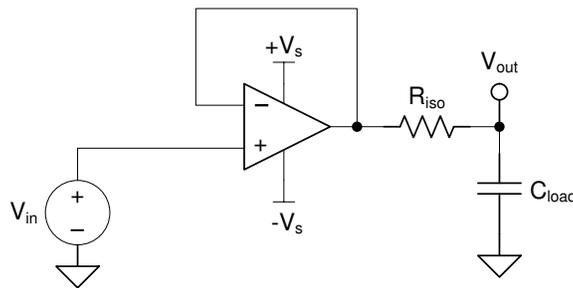
**Figure 7-6. Extending Capacitive Load Drive With the TLV9101**
