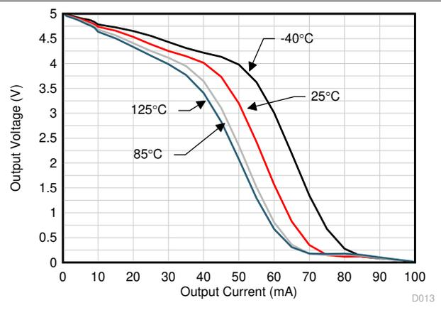
$V_S = 5\text{ V}$ ,  $R_L$  connected to  $V_-$
