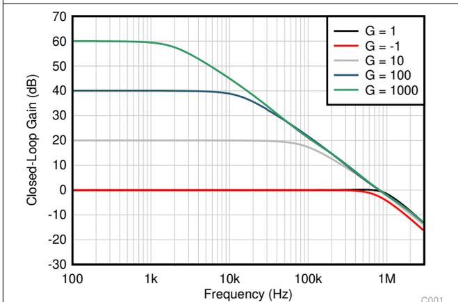
**Figure 6-11. Closed-Loop Gain and Phase vs Frequency**
