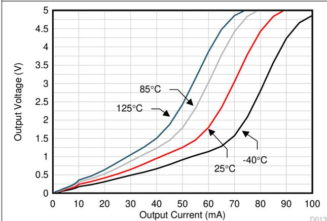
$V_S = 5\text{ V}$ ,  $R_L$  connected to  $V_+$
