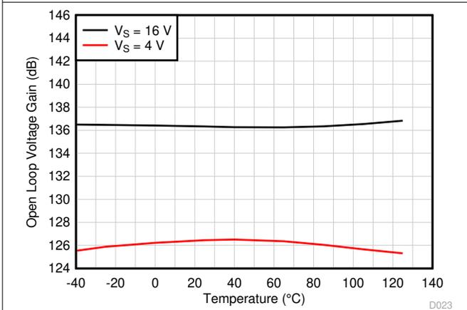
**Figure 6-27. Open-Loop Voltage Gain vs Temperature (dB)**
