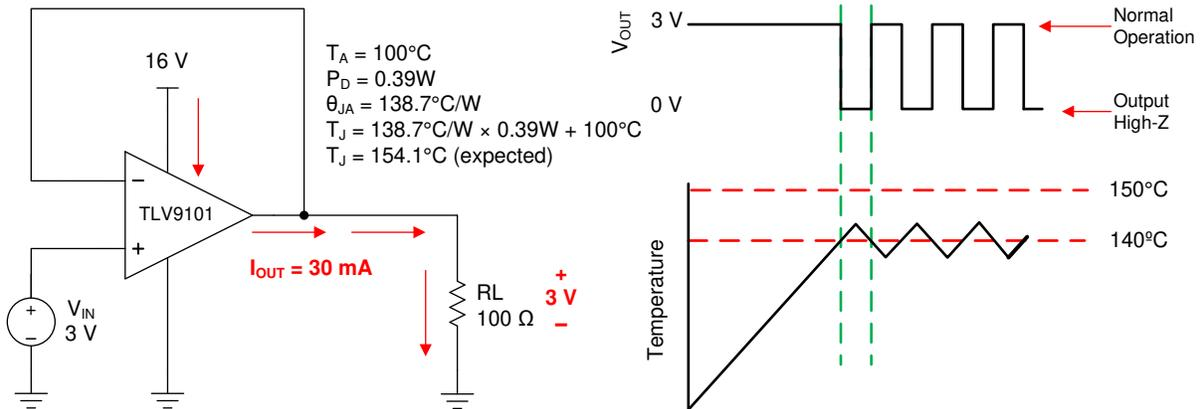
**Figure 7-3. Thermal Protection**
