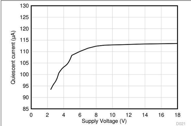
**Figure 6-25. Quiescent Current per Channel vs Supply Voltage**
