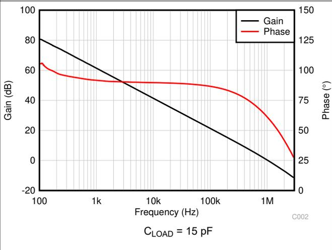
**Figure 6-10. Open-Loop Gain and Phase vs Frequency**
