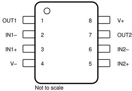
**Figure 5-4. TLV9102 D, DDF, DGK, and PW Package
