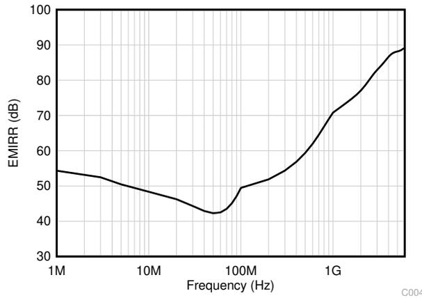
Figure 6-43. EMIRR (Electromagnetic Interference Rejection Ratio) vs Frequency
