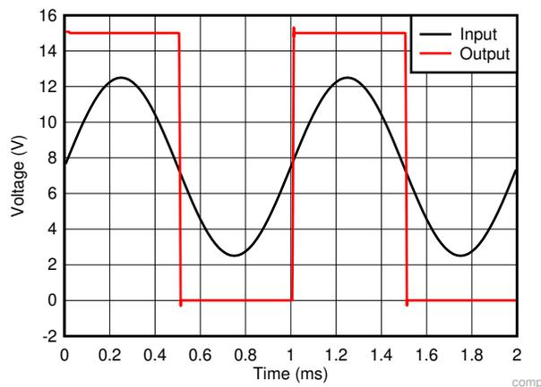
**Figure 8-2. Comparator Output Response to Input Voltage**
