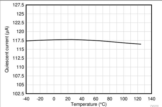
**Figure 6-26. Quiescent Current per Channel vs Temperature**
