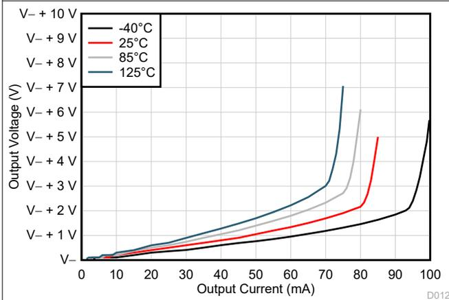
**Figure 6-15. Output Voltage Swing vs Output Current (Sinking)**
