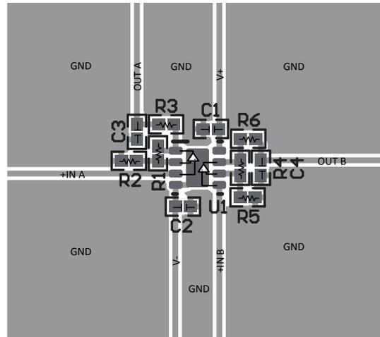
Figure 10-5. Example Layout for WSON-8 (DSG) Package
