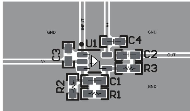
**Figure 10-3. Example Layout for SC70 (DCK) Package**
