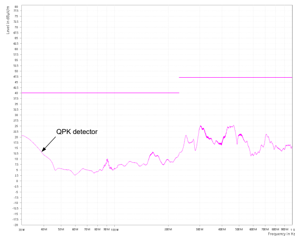
Figure 9-10. CISPR 32 Class B Radiated Emissions: Horizontal Polarization
