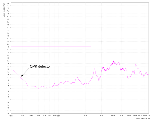
Figure 9-11. CISPR 32 Class B Radiated Emissions: Vertical Polarization
