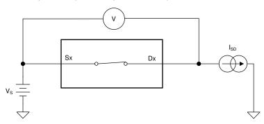
Figure 7-1. On-Resistance Measurement Setup
