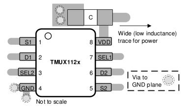
Figure 9-8. TMUX112x Layout Example
