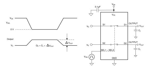
Figure 7-6. Charge-Injection Measurement Setup
