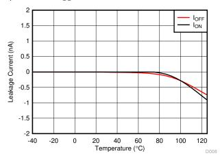
Figure 8-1. Leakage Current vs Temperature
