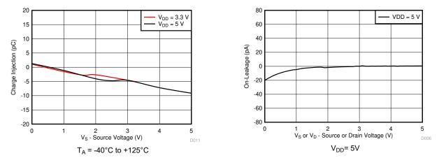
Figure 9-3. Charge Injection vs Source Voltage
