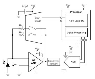
Figure 9-5. Switching Gain Settings of a TIA Circuit
