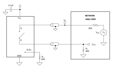
Figure 7-7. Off Isolation Measurement Setup
