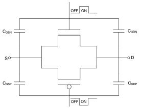
Figure 8-2. Transmission Gate Topology
