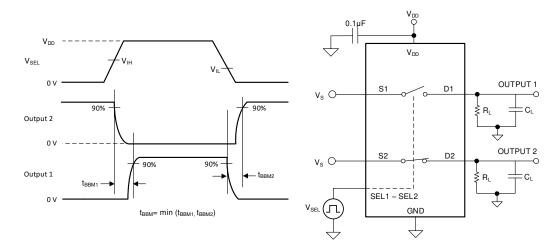
Figure 7-5. Break-Before-Make Delay Measurement Setup
