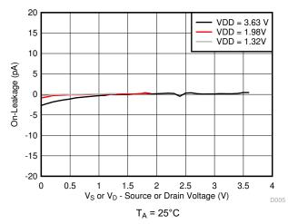
Figure 9-6. On-Leakage vs Source or Drain Voltage
