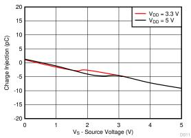
Figure 8-3. Charge Injection vs Source Voltage
