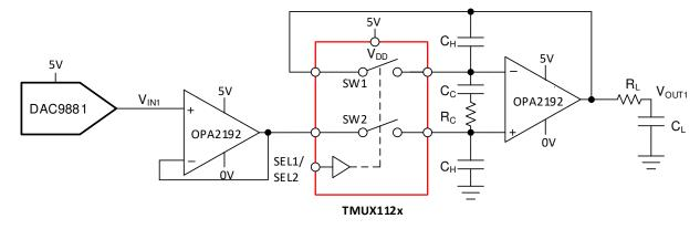
Figure 9-2. 2-Channel Sample-and-Hold Circuit with Pedestal Error Compensation
