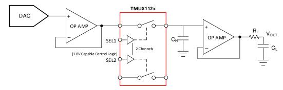
Figure 9-1. Single Channel Sample-and-Hold Circuit Example
