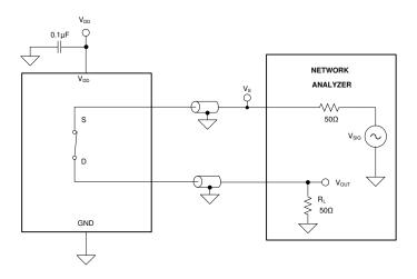
Figure 7-9. Bandwidth Measurement Setup
