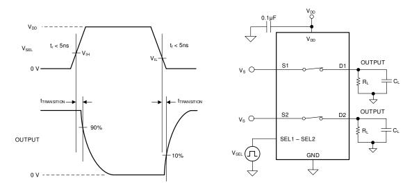
Figure 7-4. Transition-Time Measurement Setup
