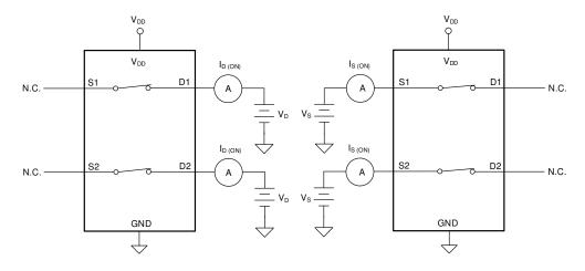
Figure 7-3. On-Leakage Measurement Setup
