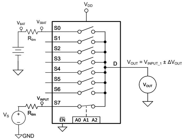
**Figure 9-3. Channel S7 selected, Channel S0 experiencing a short-to-battery condition**
