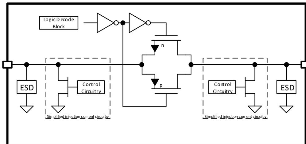
**Figure 8-3. Simplified Diagram of Injection Current Control**
