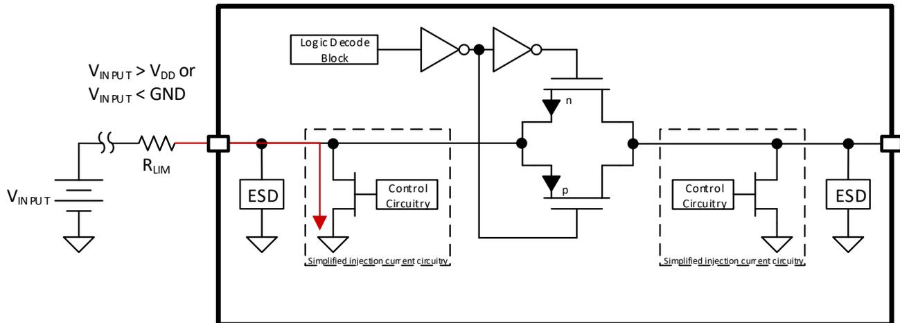
Figure 8-5. Over-Voltage Event with Series Resistor
