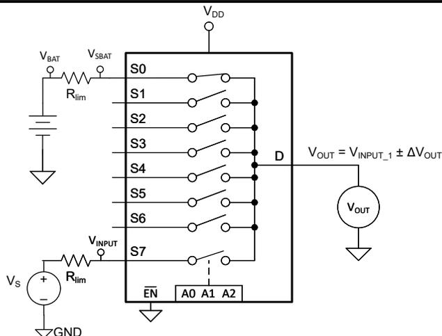
**Figure 9-5. Short-to-Battery Condition Only on a Single Selected Channel**
