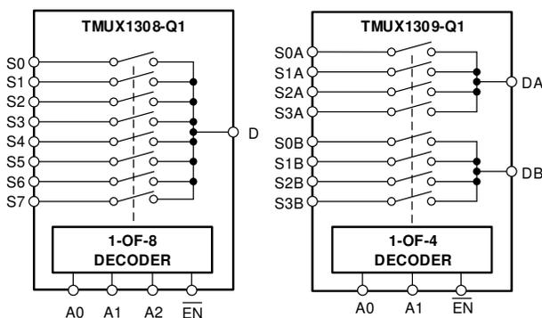
Figure 2-1. TMUX1308-Q1 and TMUX1309-Q1: Block Diagram
