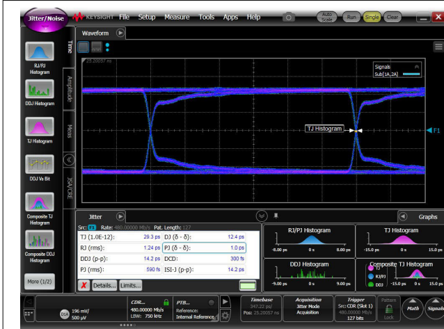
Figure 6-7. Through Calibration Traces at 480Mbps
