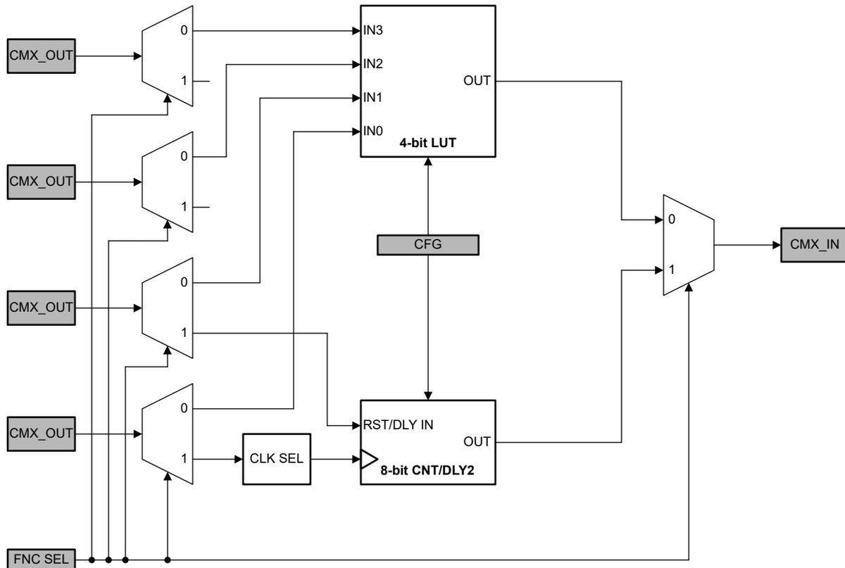
Figure 7-8. 4-bit LUT or 8-bit CNT/DLY Block Diagram
