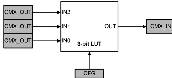
Figure 7-3. 3-bit LUT Block Diagram
