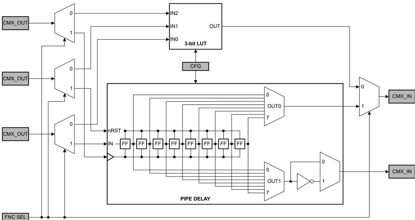
Figure 7-6. 3-bit LUT or Pipe delay block diagram
