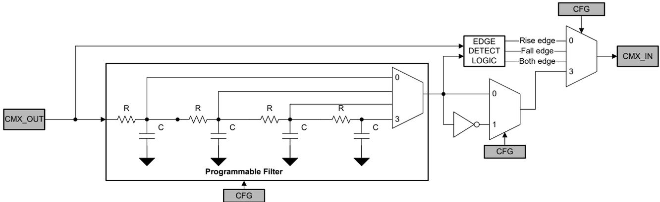
**Figure 7-17. Programmable Filter and Edge Detector Block Diagram**
