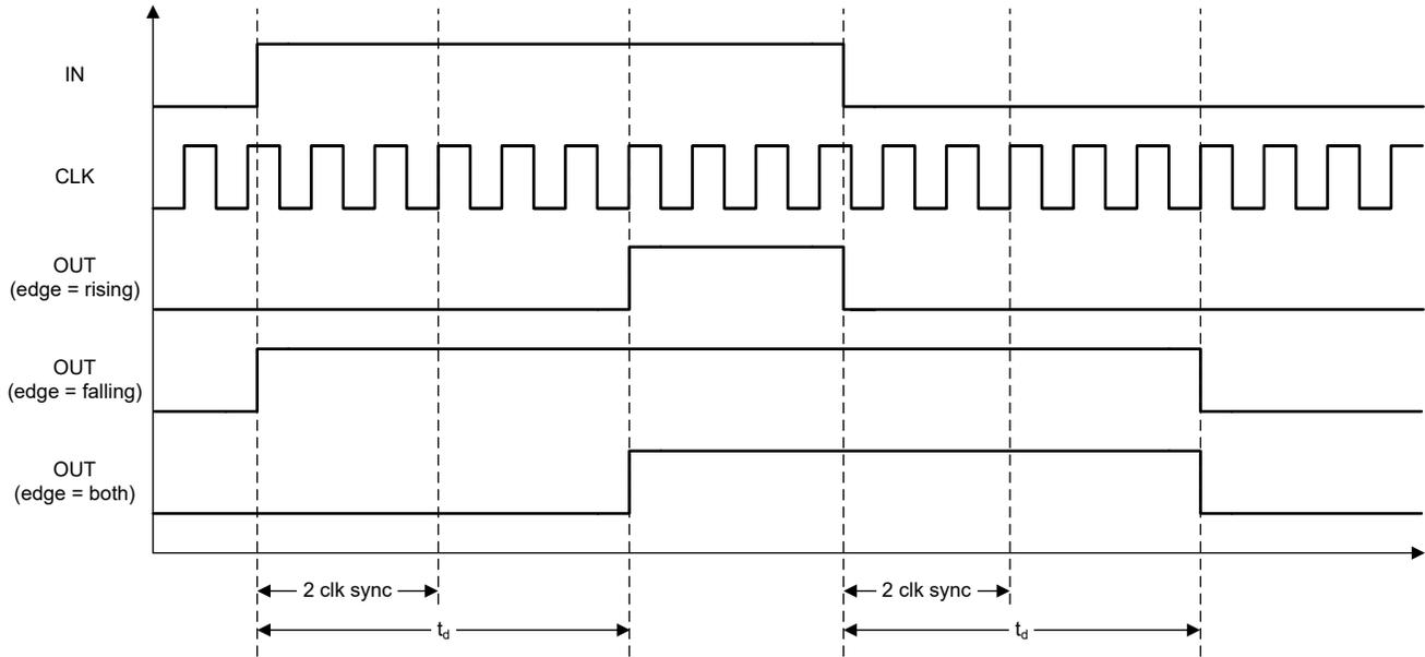
Figure 7-12. Delay Output Timing Example (DATA = 3)
