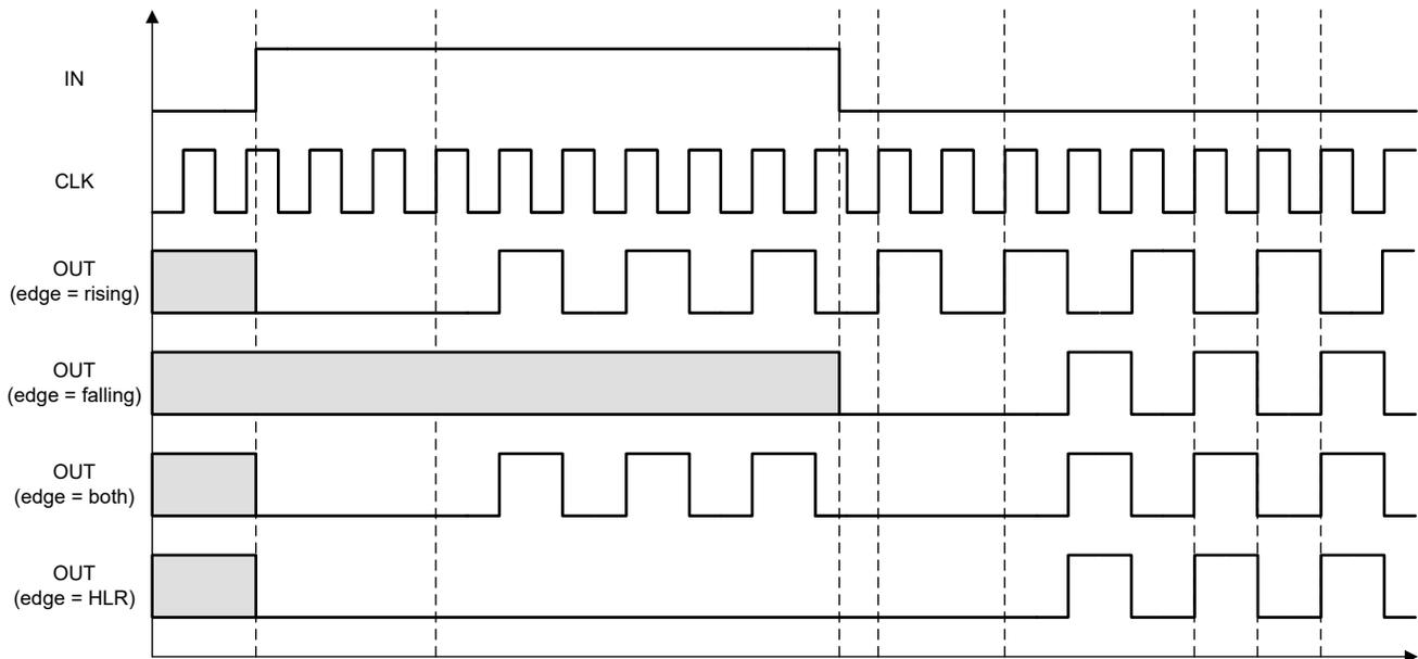
**Figure 7-14. Counter Output Timing Example (DATA = 1)**
