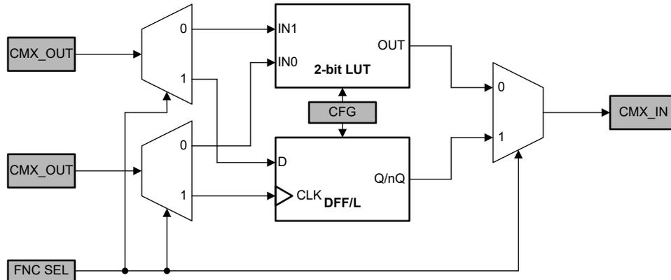
Figure 7-4. 2-bit LUT or DFF/Latch Block Diagram
