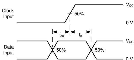
**Figure 6-5. Voltage Waveforms, Setup and Hold Times**
