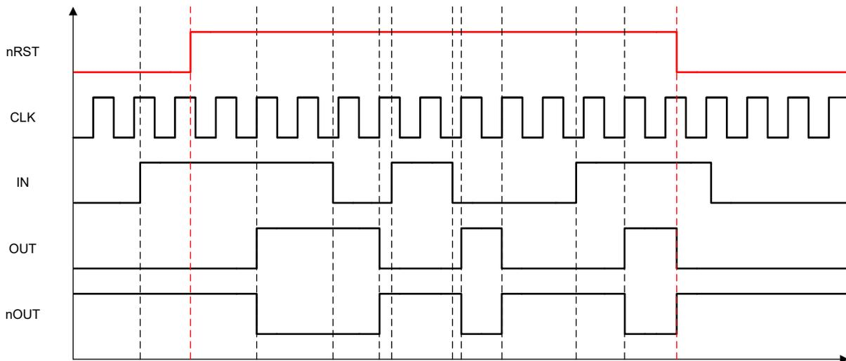
**Figure 7-7. Pipe Delay Macro-Cell Timing Example (Delay = 2)**
