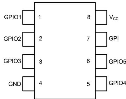
**Figure 4-1. DRL Package, 8-pin SOT-5X3 (Top View)**
