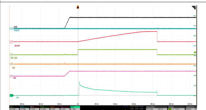
Figure 8-7. Power Up Into Short: V_{IN} = 54V , EN/UVLO Stepped Up From 0V to 3V
