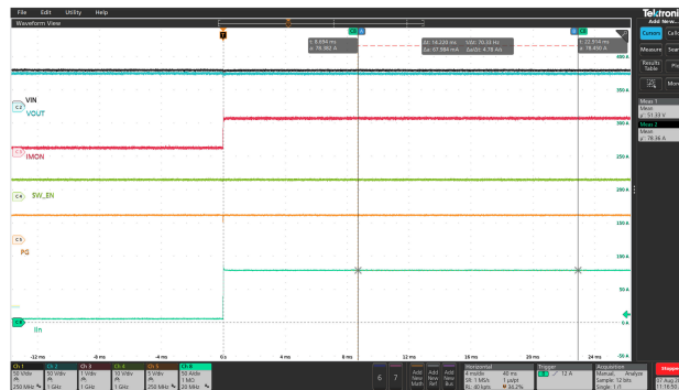
Figure 7-6. Analog Load Current Monitor Response
