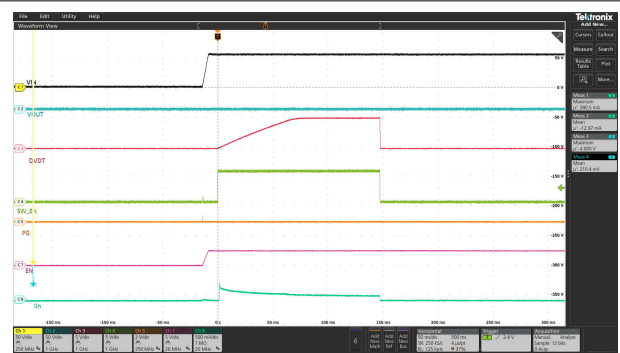
Figure 6-8. Power Up into Short-Circuit
