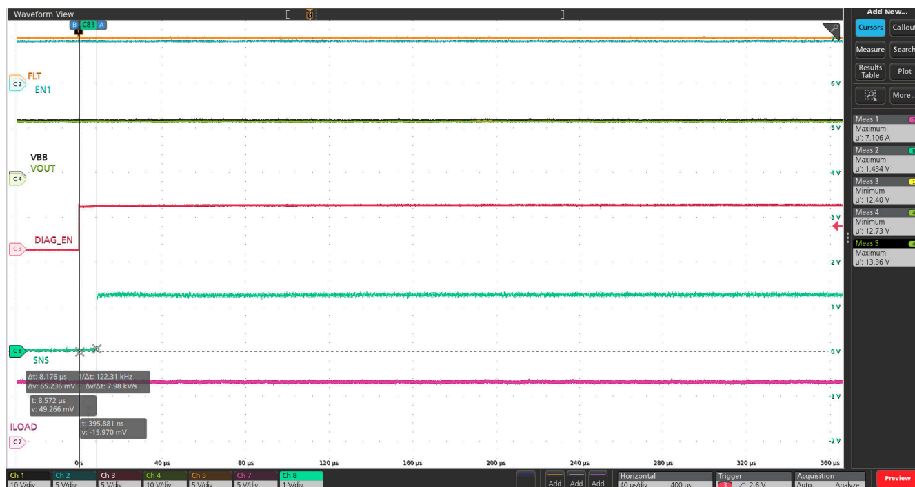
Figure 8-5. SNS Response Time with DIAG_EN ( t_{SNSION1} )
