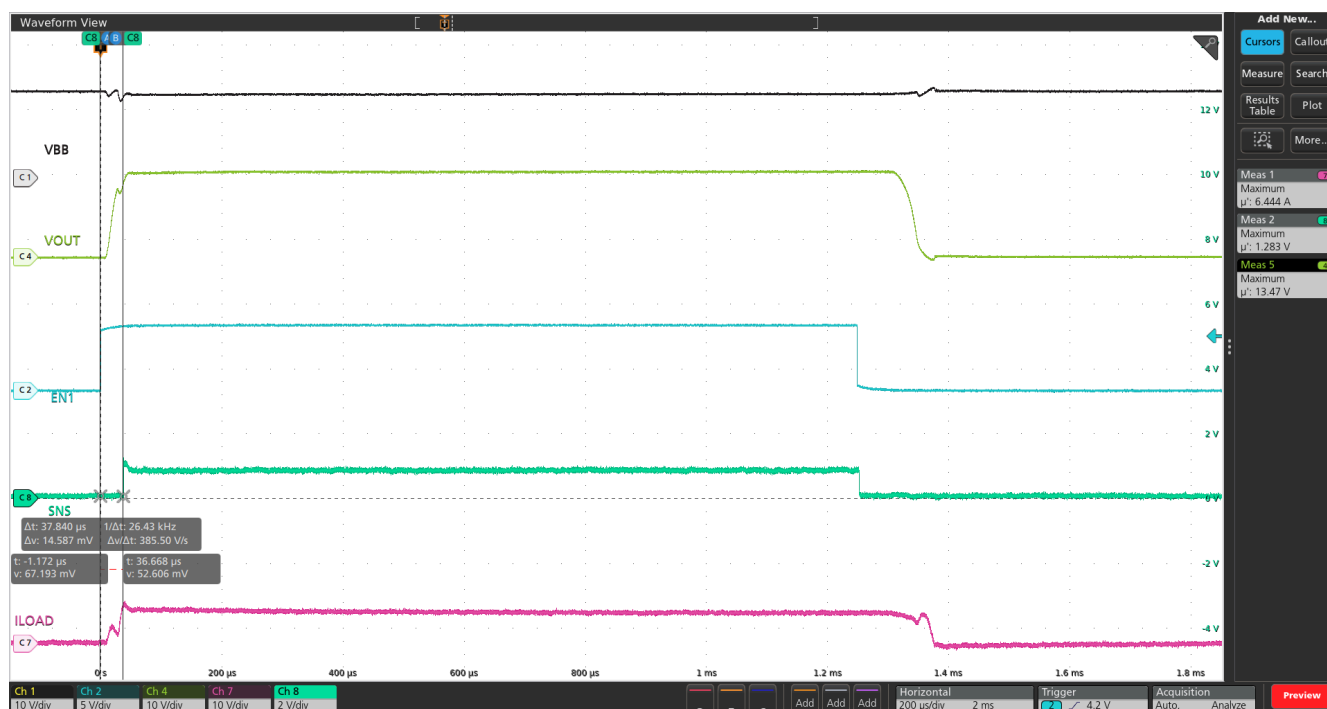
Figure 8-6. SNS Response Time with EN ( t_{SNSION3} )
