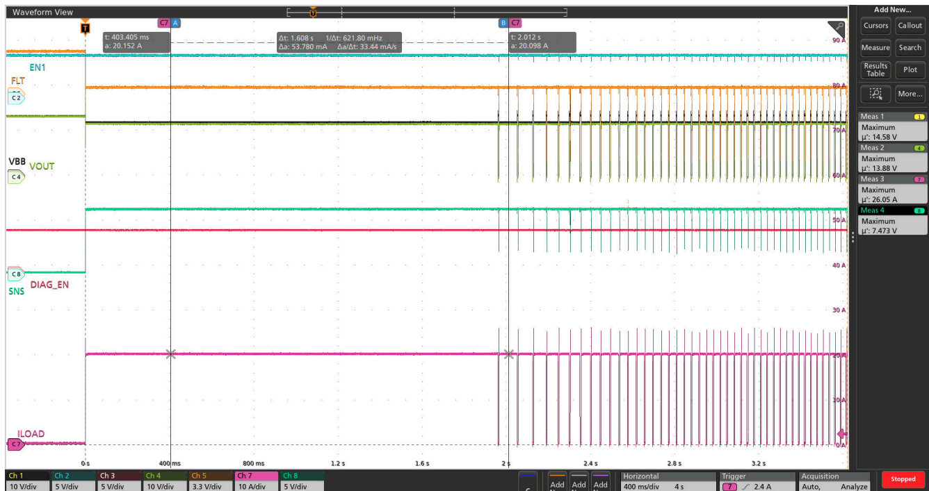
Figure 8-18. Device Enters Into Infinite Thermal Shutdown Retry Phase For Load Current (20A electronic load) Less Than Current Limit (ILIM = GND)
