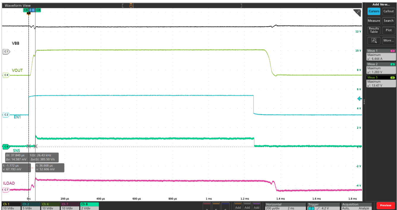
Figure 8-6. SNS Response Time with EN ( t_{SNSION3} )
