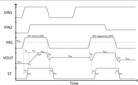
Figure 7-1. Priority and Manual Mode Switching
