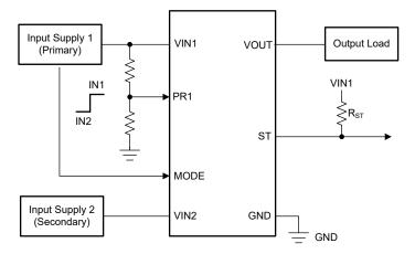
Figure 8-1. TPS2117 Typical Application Diagram
