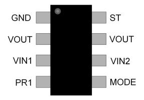
Figure 5-1. DRL Package, 8-Pin SOT (Top View)
