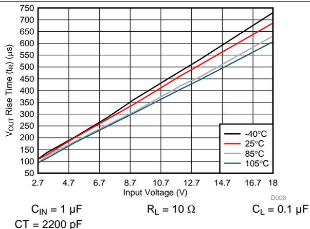
Figure 7.  $V_{OUT}$  Rise Time ( $t_R$ ) vs Input Voltage
