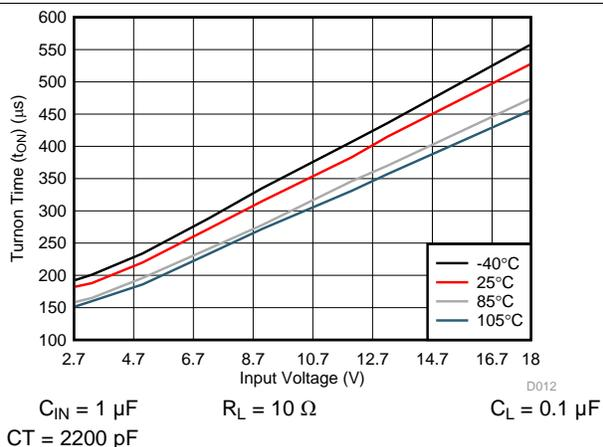
Figure 11. Turnon Time ( $t_{ON}$ ) vs Input Voltage
