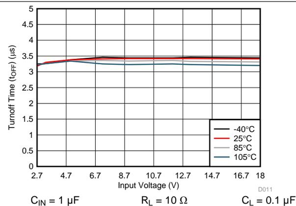
Figure 10. Turnoff Time ( $t_{OFF}$ ) vs Input Voltage
