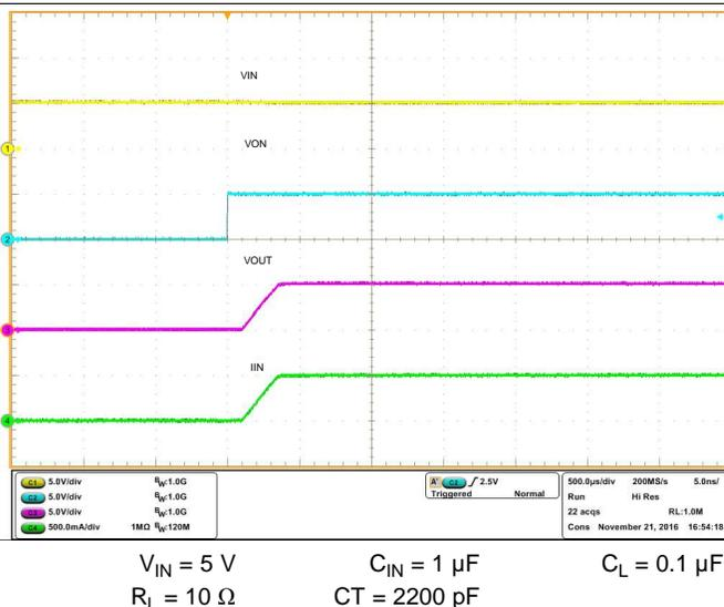
Figure 12. Rise Time  $t_R$  at  $V_{IN} = 5\text{ V}$
