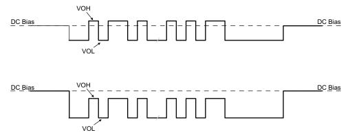
Figure 8-23. TX Driver Transmission with DC Bias
