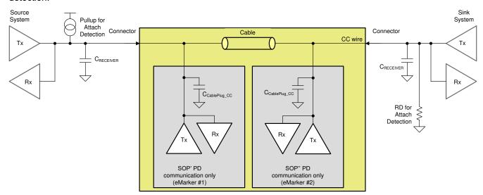
Figure 8-25. Example USB-PD Multi-Drop Configuration
