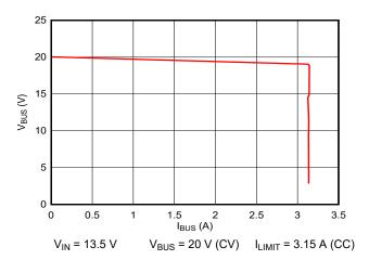
Figure 6-32. Constant Voltage to Constant Current Transition
