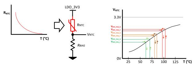
Figure 8-43. NTC Response Curve
