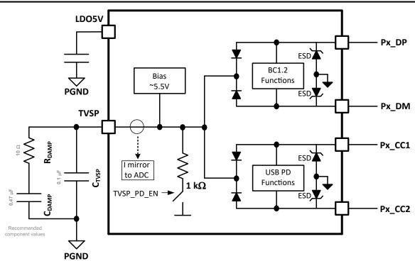
Figure 8-4. Basic TVSP Pin Connection
