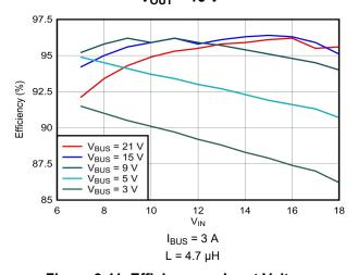
Figure 9-11. Efficiency vs Input Voltage
