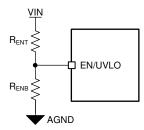
Figure 8-2. UVLO Threshold Programming
