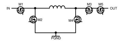
Figure 8-7. Buck-Boost Internal Power FETs
