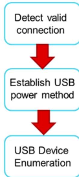
Figure 8. DFP to UFP Connect Flow
