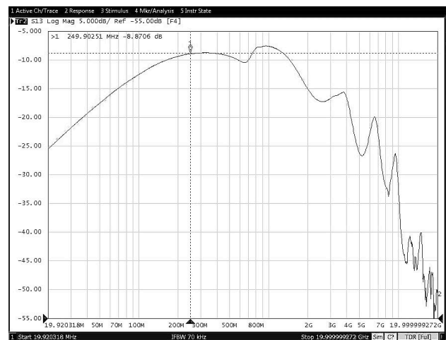
Figure 8-24. Off-state Data-Switch Isolation vs Frequency
