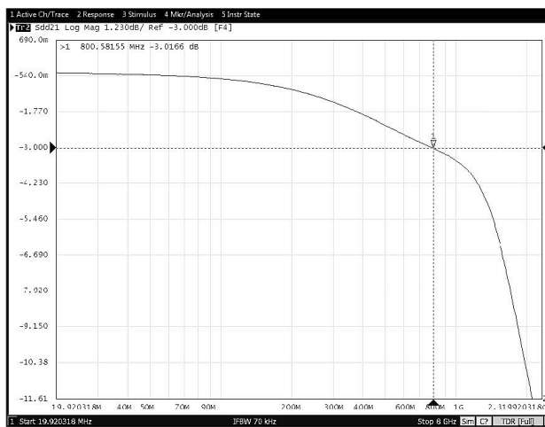
Figure 8-23. Data Transmission Characteristics vs Frequency
