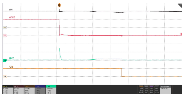
V_{IN} = 12V , R_{ILM} = 649\Omega , OUT stepped from Open \rightarrow Short-circuit to GND
