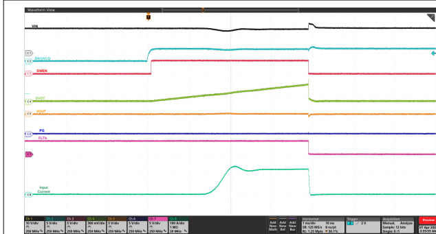
Figure 9-8. Power Up into Short: V_{IN} = 12 V, EN/UVLO Stepped Up From 0 V to 3 V, R_{REF} = 40.2 k \Omega , R_{ILIM} on Each Device = 442 \Omega , and OUT Shorted to GND
