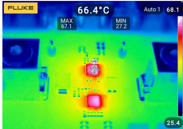
Figure 9-12. Two Devices in Parallel Temperature Rise with 110-A DC Current at Room Temperature (No Air-Flow)
