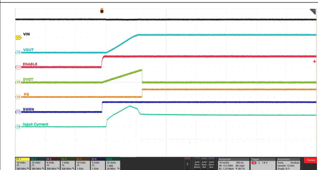
Figure 7-28. Inrush Current Control with Capacitive and Resistive Load
