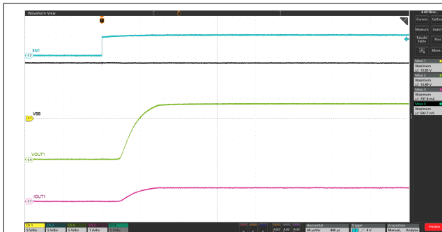
Figure 9-3. Turn-on with Resistive Load
