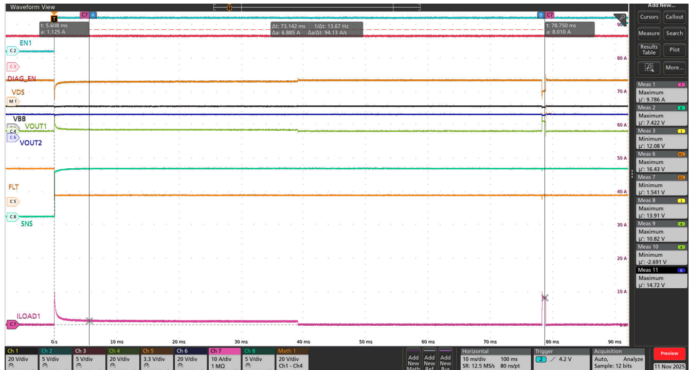
Figure 8-23. Device Entering Into Extended Retry Window with Thermal Regulation Behavior in Initial Retry Window
