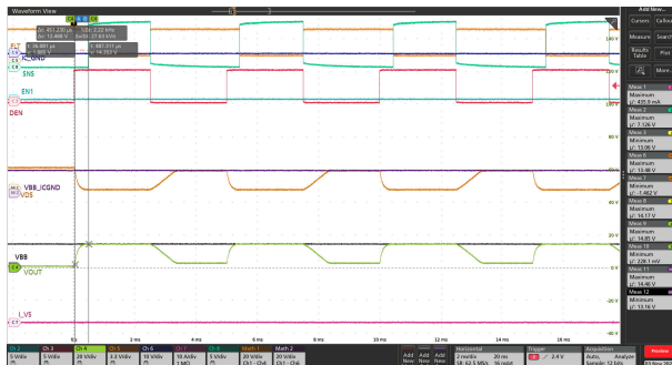
Figure 9-7. Device Turn-on Behavior with Channel 1 Output Shorted to GND
