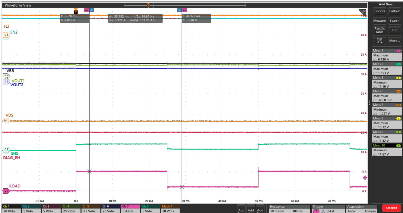
Figure 8-4. SNS Pin Voltage with Varying Load Current on Channel 1 ( R_{SNS} = 1k\Omega , SEL = 0 )
