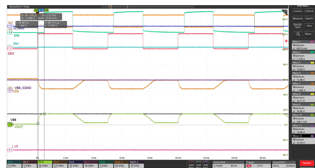
Figure 9-8. Falling Slew Rate (P, M version)
