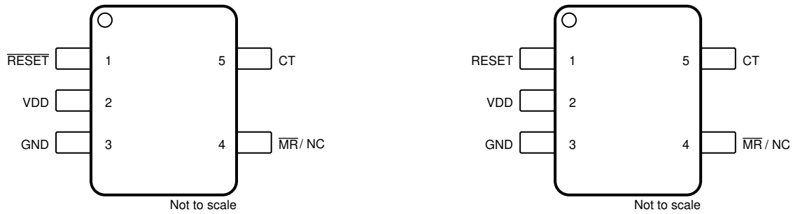
Figure 5-1. DBV Package 5-Pin SOT-23 TPS3840PL, Figure 5-2. DBV Package 5-Pin SOT-23 TPS3840PH Top View
