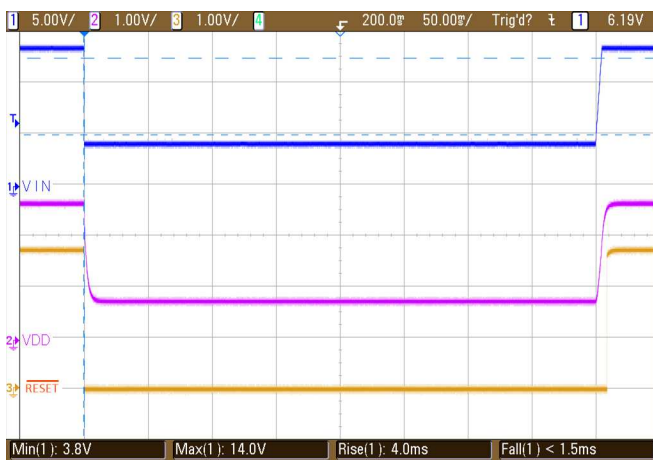
Figure 51. TPS3840-Q1 Warm-Start Test Pulse
