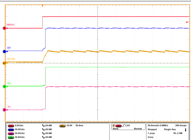
Figure 8-3. Start-Up Profile of Bootstrap Voltage with INP = HIGH and C_{BST} = 470nF
