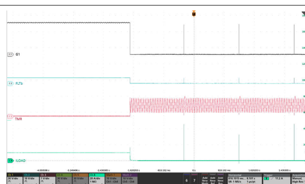
Figure 8-7. Auto-Retry Response of TPS48130-Q1 for an Overcurrent Fault
