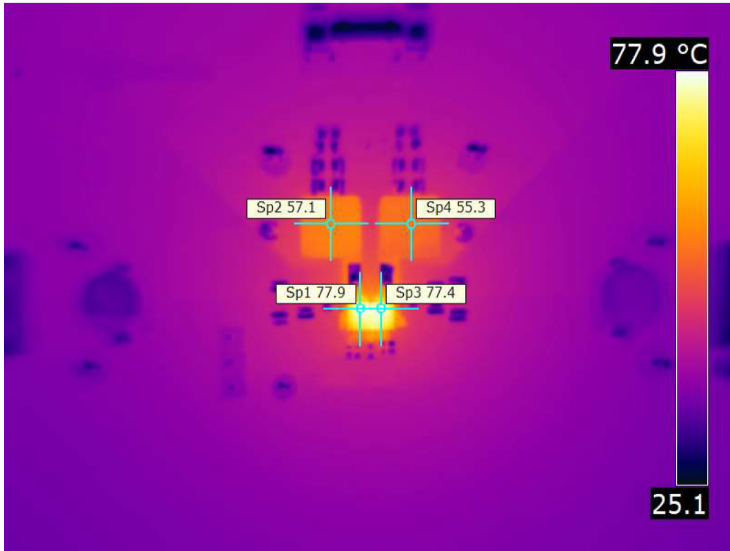
Figure 10-4. Thermal Image at 25°C Ambient - Dual Output Operation, f_{sw} = 1 \text{ MHz} , V_{IN} = 12 \text{ V} , V_{OUT1} = 1 \text{ V} , I_{OUT1} = 6 \text{ A} , L_1 = 560 \text{ nH} (3.3 m \Omega Max), V_{OUT2} = 3.3 \text{ V} , I_{OUT2} = 6 \text{ A} , L_2 = 1.2 \text{ }\mu\text{H} (7.5 m \Omega Max)
