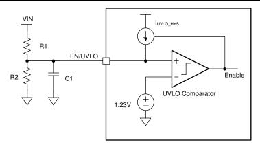
Figure 7-1. Programmable UVLO With Resistor Divider at the EN/UVLO Pin
