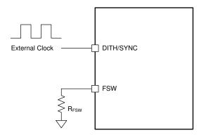
Figure 7-3. External Clock Configuration
