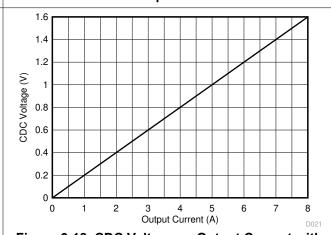
Figure 6-18. CDC Voltage vs Output Current with  $R_{SENSE}$  = 10  $m\Omega$
