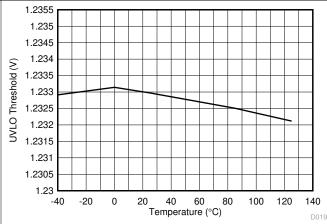
Figure 6-16. ENABLE/UVLO Rising Threshold vs Temperature
