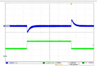
Figure 8-11. Load Transient Waveforms in  $V_{\text{IN}}$  = 12 V,  $V_{\text{OUT}}$  = 5 V,  $I_{\text{O}}$  = 2.5 A to 5 A with 20- $\mu$ s Slew Rate, FPWM
