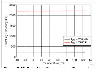
Figure 6-17. Switching Frequency vs Temperature
