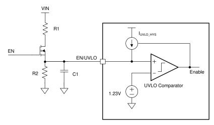
Figure 7-2. Logic Enable and Programmable UVLO
