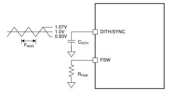
Figure 7-4. Switching Frequency Dithering
