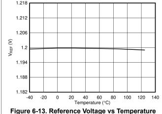
Figure 6-13. Reference Voltage vs Temperature (V<sub>REF</sub> = 1.2 V)
