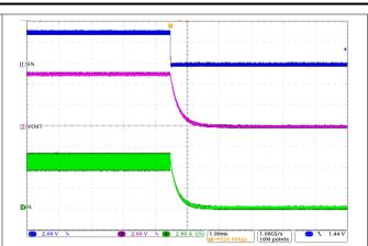
Figure 8-9. Shutdown Waveforms in  $V_{IN}$  = 12 V,  $V_{OUT}$  = 5 V,  $I_{O}$  = 5 A, FPWM
