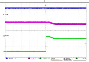
Figure 8-12. Output Current Limit Waveforms in  $V_{IN}$  = 12 V,  $V_{OUT}$  = 5 V,  $R_{LOAD}$  = 0.9  $\Omega$ ,  $R_{SNS}$  = 10 m $\Omega$ , FPWM
