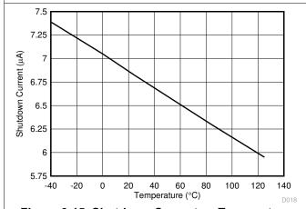
Figure 6-15. Shutdown Current vs Temperature
