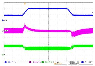
Figure 8-10. Line Transient Waveforms in  $V_{IN}$  = 9 V to 20 V,  $V_{OUT}$  = 12 V,  $I_{O}$  = 5 A with 200- $\mu$ s Slew Rate, FPWM
