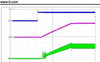
Figure 8-8. Start-up Waveforms in  $V_{IN}$  = 12 V,  $V_{OUT}$  = 5 V,  $I_O$  = 5 A, FPWM
