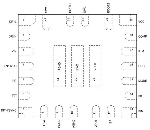
Figure 5-1. 26-pin VQFN-HR RPM Transparent (Top View)
