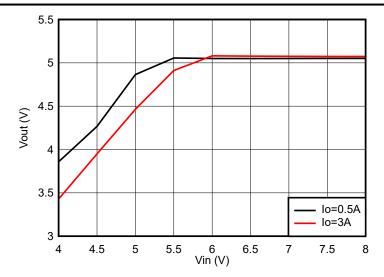
Figure 7-6. Overall Dropout Characteristic, V<sub>OUT</sub> = 5 V
