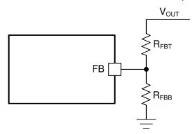
Figure 7-2. Output Voltage Setting
