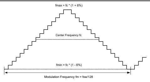
Figure 7-4. Frequency Spread Spectrum Diagram
