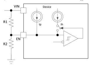
Figure 7-3. Adjustable V<sub>IN</sub> Undervoltage Lockout
