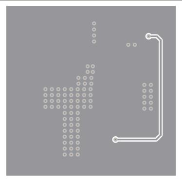
Figure 8-24. TPS563300 Bottom Layout Example
