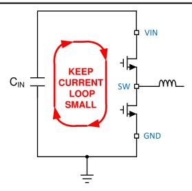
Figure 8-22. Current Loop With Fast Edges
