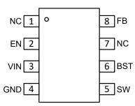
Figure 5-1. 8-Pin SOT583 DRL Package (Top View)
