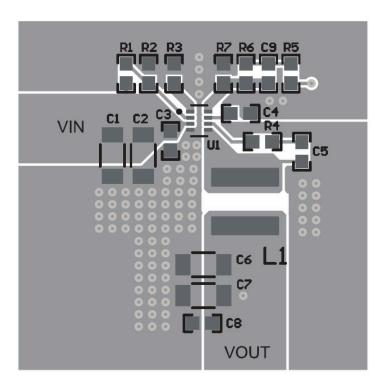
Figure 8-23. TPS563300 Top Layout Example
