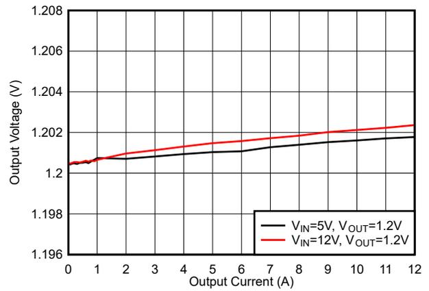
Figure 5-22. Load Regulation,  $F_{sw} = 800 \text{ kHz}$
