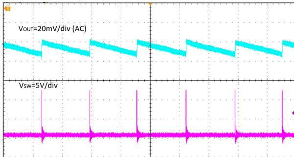
Figure 7-4. Output Voltage Ripple,  $I_{OUT} = 10\text{ mA}$ ,
