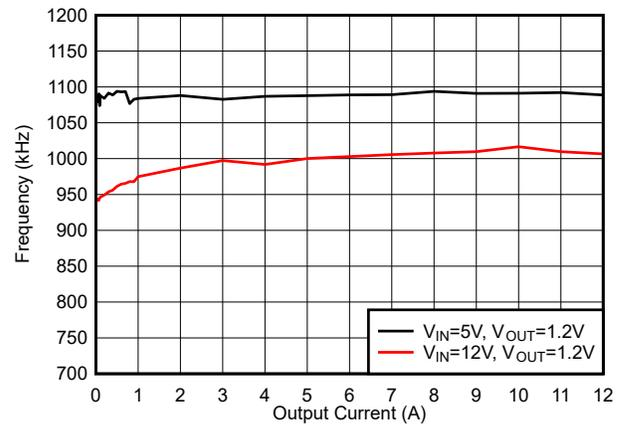
Figure 5-28.  $F_{SW}$  Load Regulation, Mode = FCCM,  $F_{SW} = 1200$  kHz
