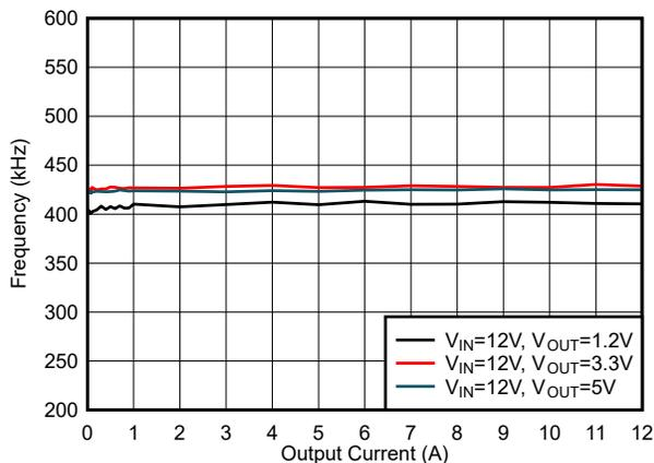
Figure 5-29.  $F_{SW}$  Load Regulation, Mode = FCCM,  $F_{SW} = 400$  kHz
