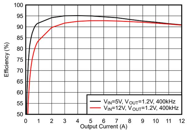
Figure 5-10. Efficiency, FCCM Mode,  $f_{sw} = 400 \text{ kHz}$
