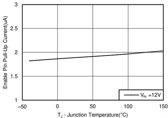
**Figure 5-5. Enable Pullup Current, V<sub>EN</sub> = 1.0 V**
