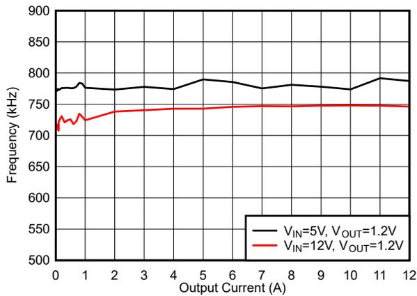
Figure 5-27.  $F_{SW}$  Load Regulation, Mode = FCCM,  $F_{SW} = 800$  kHz
