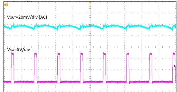
Figure 7-5. Output Voltage Ripple,  $I_{OUT} = 12\text{ A}$ ,
