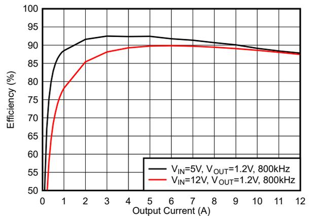
Figure 5-12. Efficiency, FCCM Mode,  $f_{sw} = 800 \text{ kHz}$
