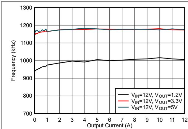
Figure 5-31.  $F_{SW}$  Load Regulation, Mode = FCCM,  $F_{SW} = 1200$  kHz
