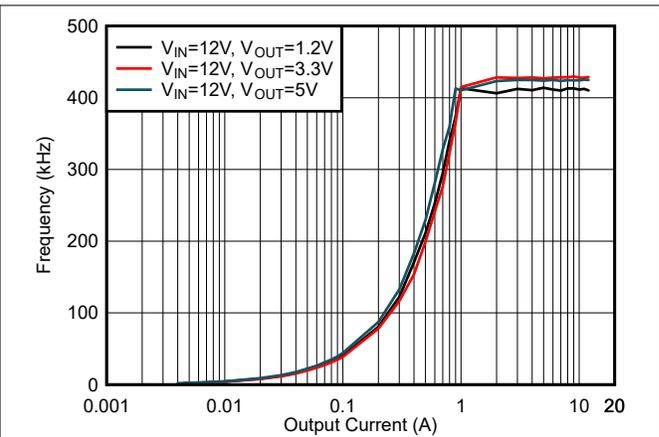
Figure 5-32.  $F_{SW}$  Load Regulation, Mode = DCM,  $F_{SW} = 400$  kHz
