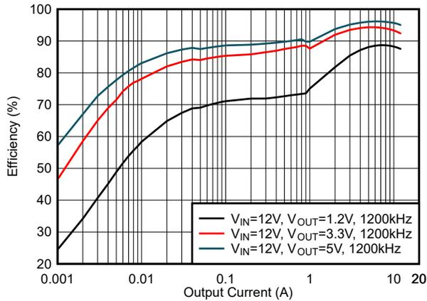
Figure 5-19. Efficiency, DCM Mode,  $f_{sw} = 1200 \text{ kHz}$
