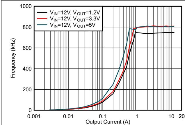
Figure 5-33.  $F_{SW}$  Load Regulation, Mode = DCM,  $F_{SW} = 800$  kHz
