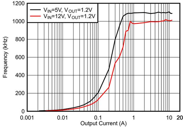
Figure 5-25.  $F_{SW}$  Load Regulation, Mode = DCM,  $F_{SW} = 1200$  kHz
