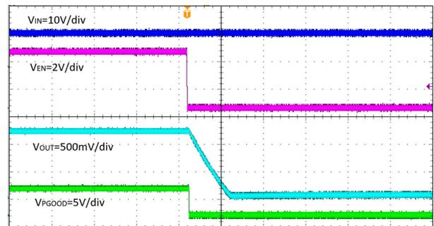
Figure 7-7. Shutdown Relative to EN Falling, Time
