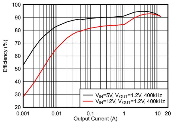
Figure 5-9. Efficiency, DCM Mode,  $f_{sw} = 400 \text{ kHz}$
