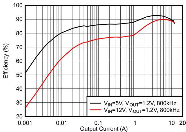
Figure 5-11. Efficiency, DCM Mode,  $f_{sw} = 800 \text{ kHz}$
