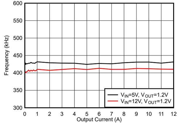
Figure 5-26.  $F_{SW}$  Load Regulation, Mode = FCCM,  $F_{SW} = 400$  kHz
