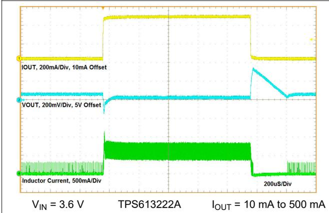
**Figure 8-16. Load Transient**
