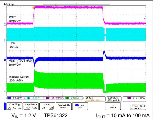
Figure 8-7. Load Transient
