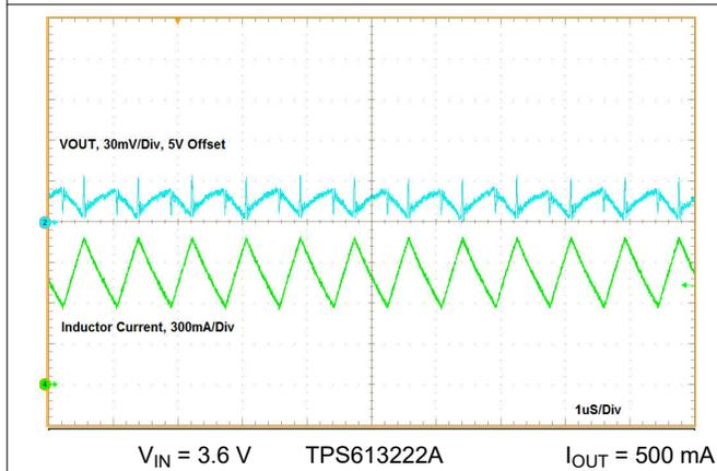
**Figure 8-12. Switching Waveform at Heavy Load**
