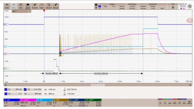
Figure 9-25. External Soft Start and Shutdown into No Load
