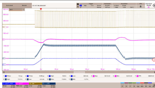
Figure 9-30. Load Transient - FPWM Operation
