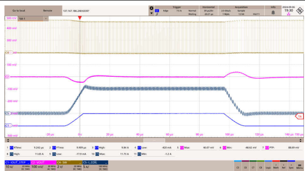
Figure 9-31. Load Transient - PFM Operation
