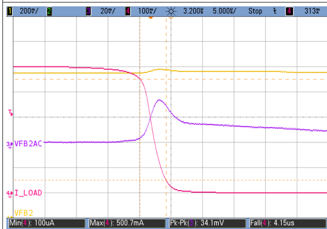
VCC2 = 3.8 V Vout = 1.2 V PWM Mode Figure 7-4. VDD2 Falling Load Transient Response
