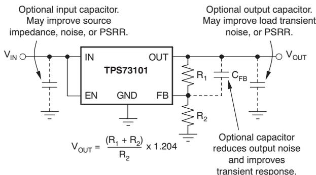
**Figure 33. Typical Application Circuit for Adjustable-Voltage Versions**
