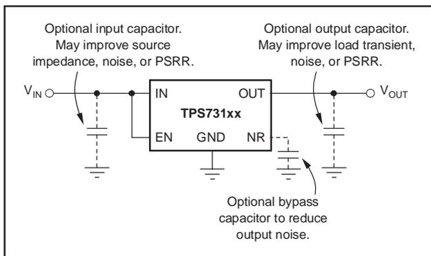
**Figure 32. Typical Application Circuit for Fixed-Voltage Versions**
