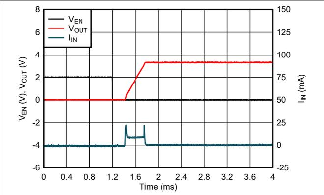
**Figure 7-7. LDO Start-Up Time With EN (New Chip)**
