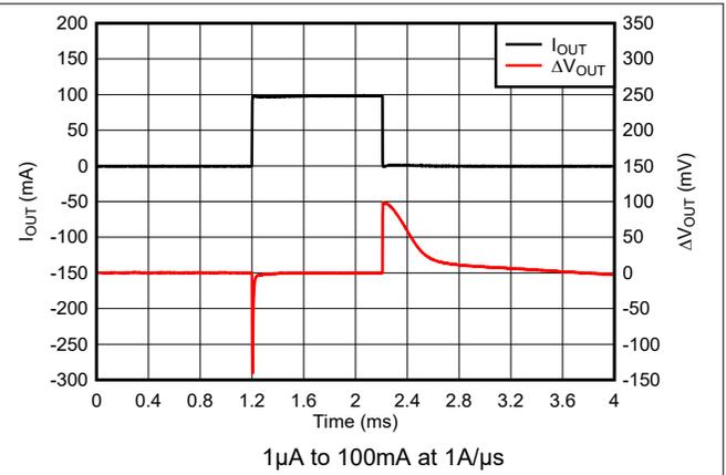
**Figure 5-44. TPS76933 Load Transient Response (New Chip)**
