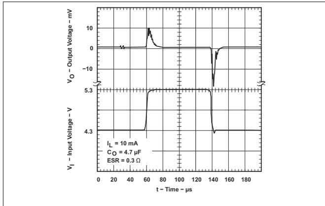
Figure 7-10. TPS76933 Line Transient Response (Legacy Chip)
