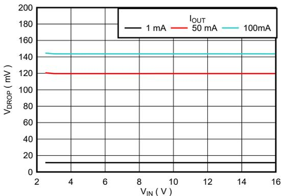
Figure 5-29. TPS76901 Dropout Voltage vs Input Supply (New Chip)
