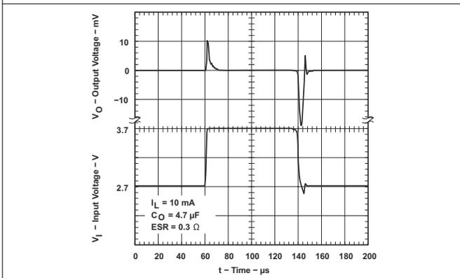
**Figure 7-8. TPS76915 Line Transient Response (Legacy Chip)**
