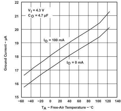
Figure 5-12. TPS76933 Ground Current vs Free-Air Temperature (Legacy Chip)
