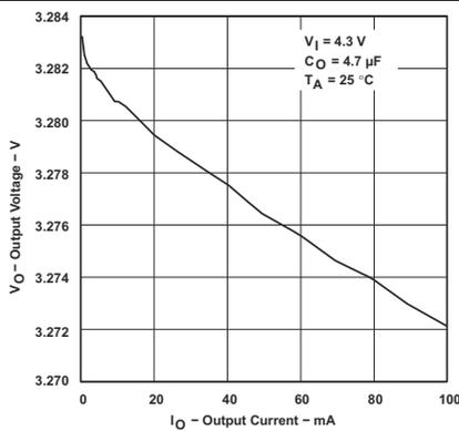
**Figure 5-3. TPS76933 Output Voltage vs Output Current (Legacy Chip)**
