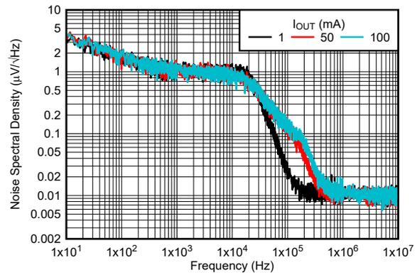
Figure 5-22. TPS76933 Output Spectral Noise Density vs Output Current (New Chip)
