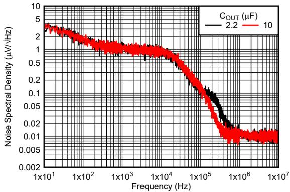
Figure 5-23. TPS76933 Output Spectral Noise Density vs Output Capacitor (New Chip)
