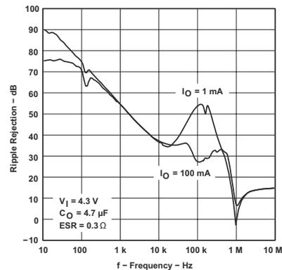
Figure 5-30. TPS76933 Ripple Rejection vs Frequency (Legacy Chip)
