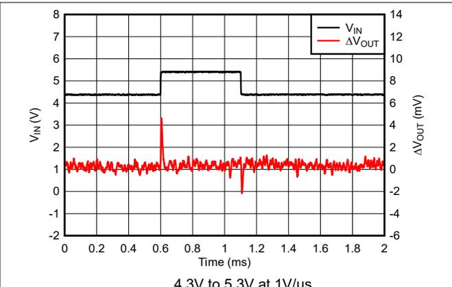
Figure 7-11. TPS76933 Line Transient Response (New Chip)
