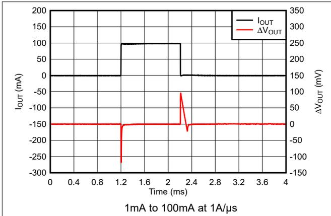
**Figure 5-43. TPS76933 Load Transient Response (New Chip)**
