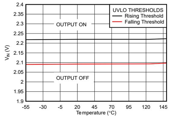
Figure 5-18. TPS76933 UVLO Threshold vs Free-Air Temperature (New Chip)
