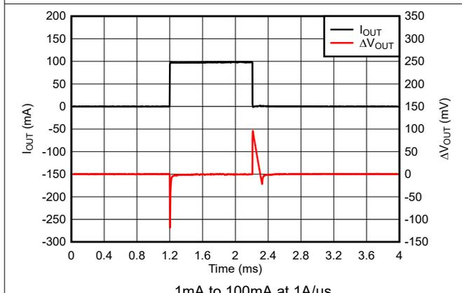
Figure 7-14. TPS76933 Load Transient Response (New Chip)
