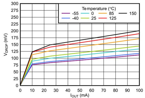
Figure 5-28. TPS76933 Dropout Voltage vs Output Current (New Chip)
