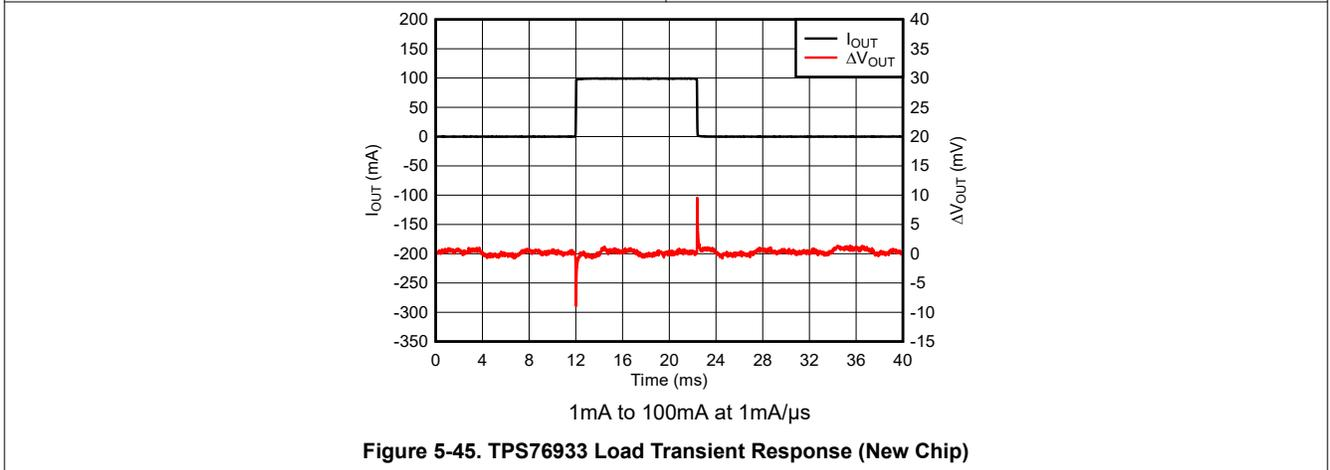
**Figure 5-45. TPS76933 Load Transient Response (New Chip)**
