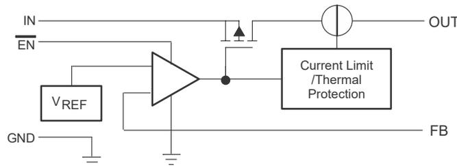
Figure 6-1. TPS76901 Functional Block Diagram (Legacy Chip)
