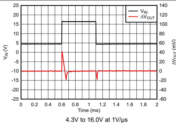
Figure 5-41. TPS76933 Line Transient Response (New Chip)
