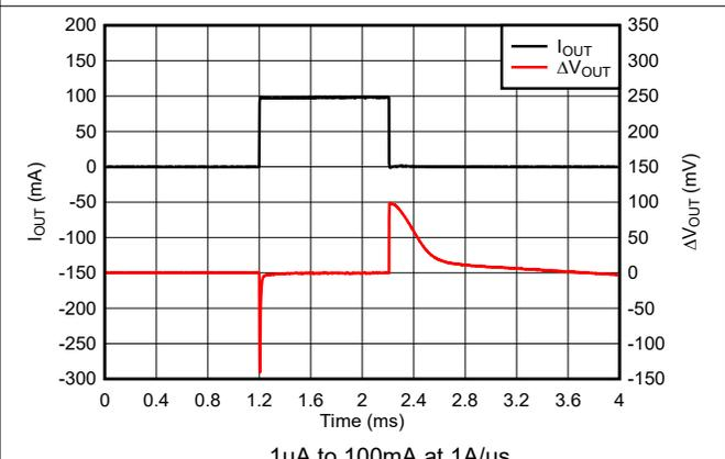
Figure 7-15. TPS76933 Load Transient Response (New Chip)
