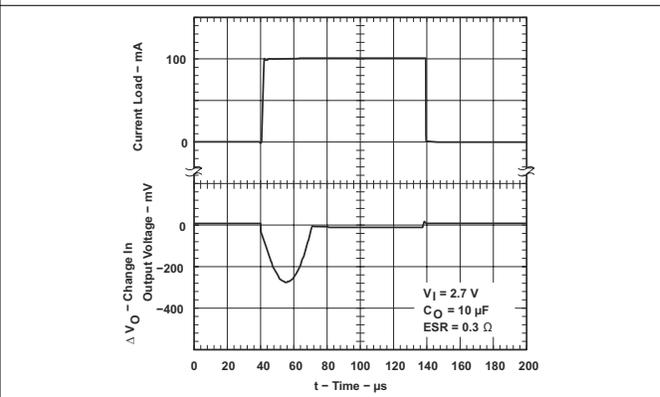
**Figure 7-9. TPS76915 Load Transient Response (Legacy Chip)**
