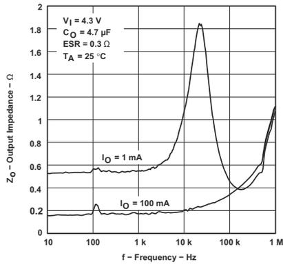
Figure 5-25. Output Impedance vs Frequency (Legacy Chip)
