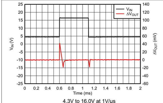
Figure 7-12. TPS76933 Line Transient Response (New Chip)
