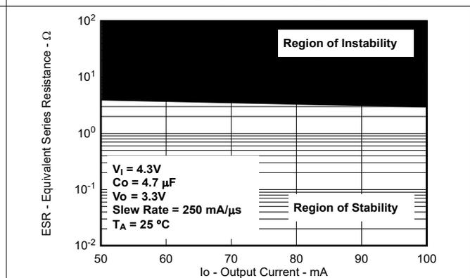
Figure 5-51. Typical Region of Stability ESR vs Output Current (New Chip)
