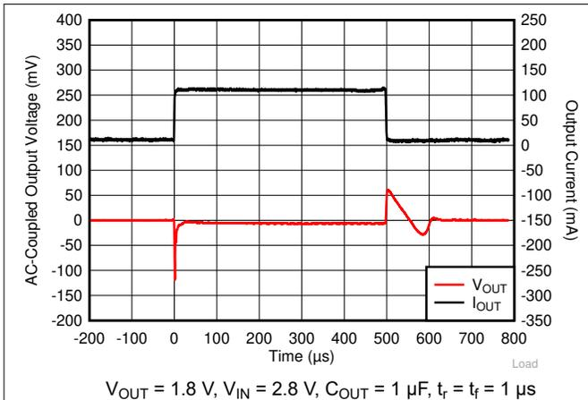
**Figure 6-13.  $I_{OUT}$  Transient From 1 mA to 100 mA**
