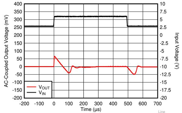
$V_{OUT} = 1.8\text{ V}$ ,  $I_{OUT} = 1\text{ mA}$ ,  $C_{OUT} = 1\text{ }\mu\text{F}$ , slew rate =  $1\text{ V}/\mu\text{s}$
