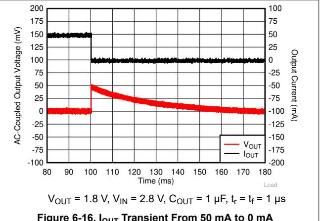
**Figure 6-16.  $I_{OUT}$  Transient From 50 mA to 0 mA**
