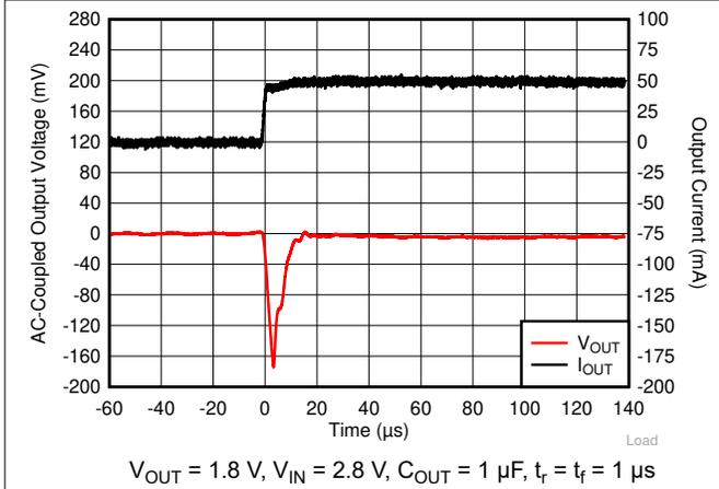
**Figure 6-15.  $I_{OUT}$  Transient From 0 mA to 50 mA**
