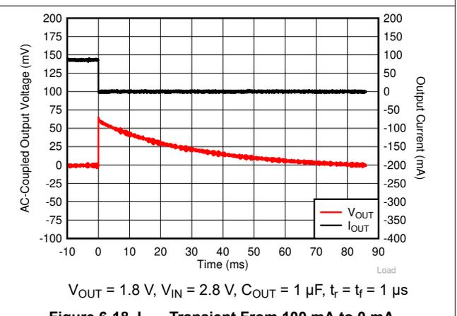
**Figure 6-18.  $I_{OUT}$  Transient From 100 mA to 0 mA**
