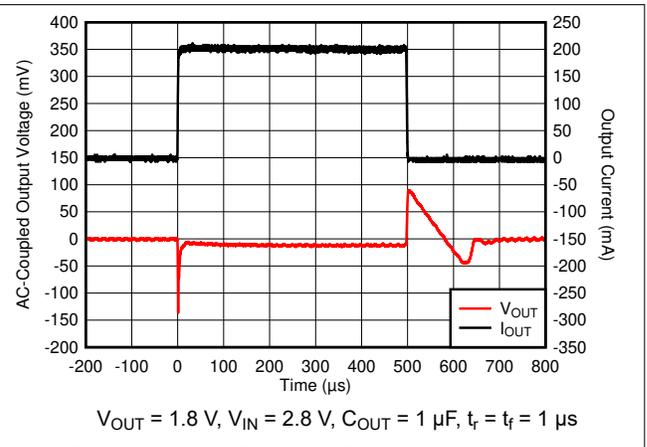
**Figure 6-14.  $I_{OUT}$  Transient From 1 mA to 200 mA**
