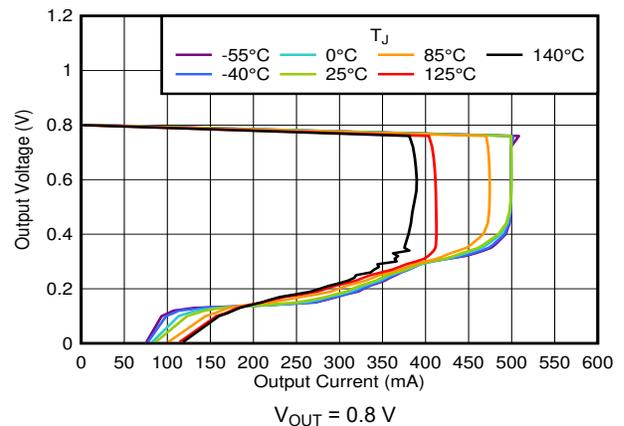
**Figure 6-36. Foldback Current Limit vs  $I_{OUT}$  and Temperature**
