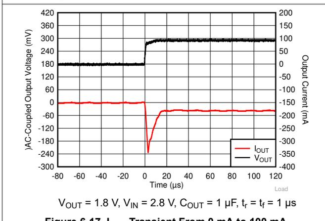
**Figure 6-17.  $I_{OUT}$  Transient From 0 mA to 100 mA**
