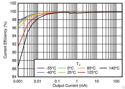
Figure 8-5. Current Efficiency vs  $I_{OUT}$  and Temperature
