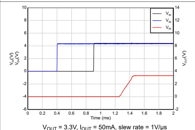
**Figure 7-9. Start-up with Sequencing (IN after EN)**
