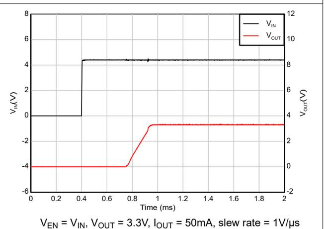
Figure 5-52. Start-up with IN and EN Tied Together
