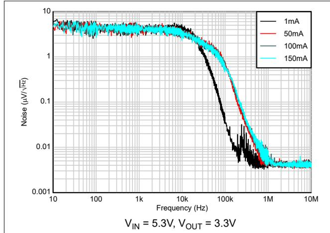
Figure 5-25. Output Noise vs Frequency, Output Current
