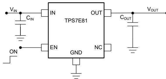
**Figure 7-4. TPS7E81 Typical Application Circuit (Fixed-Voltage Version)**
