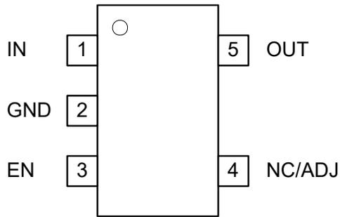
**Figure 4-1. DBV Package, (Fixed/ADJ), 5-Pin SOT-23 (Top View)**
