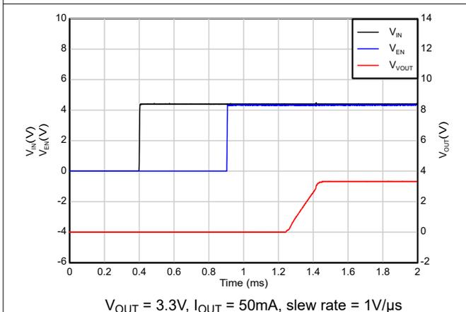
**Figure 7-8. Start-up with Sequencing (EN after IN)**
