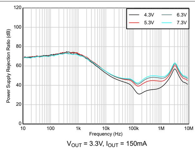
Figure 5-20. Ripple Rejection vs Frequency, Input Voltage
