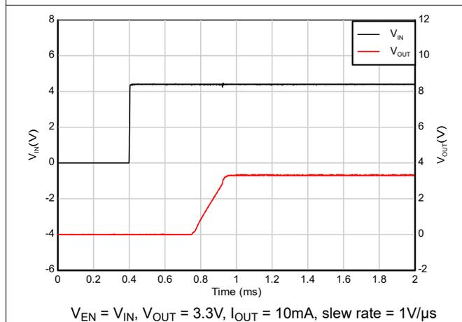
Figure 5-51. Start-up with IN and EN Tied Together
