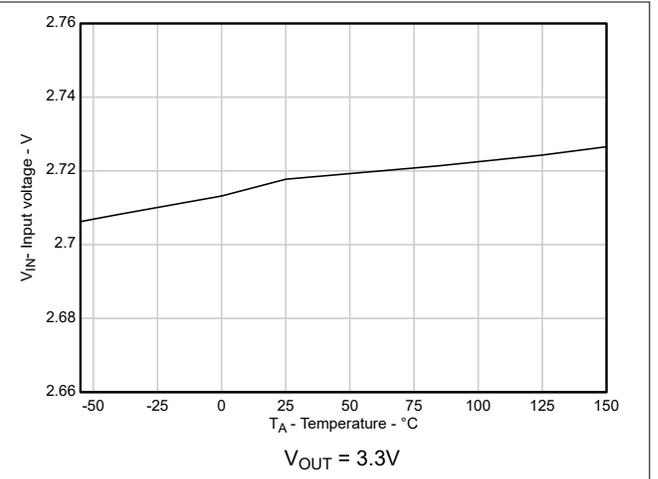
Figure 5-2. Falling Input Supply UVLO vs Temperature
