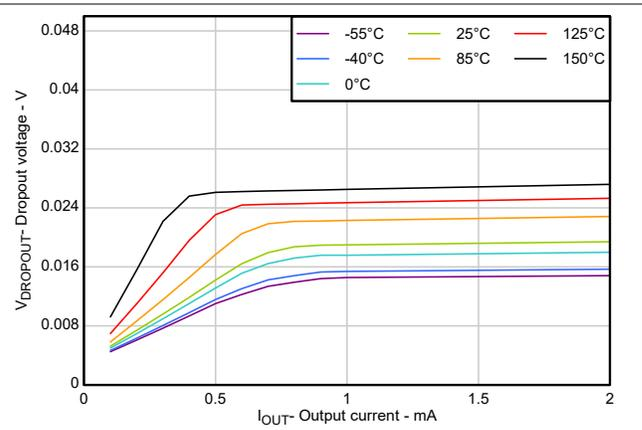
Figure 5-8. Dropout Voltage vs Output Current, Light Loads
