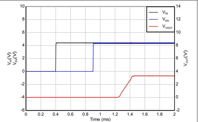
**Figure 5-46. Start-up with Sequencing (EN after IN)**
