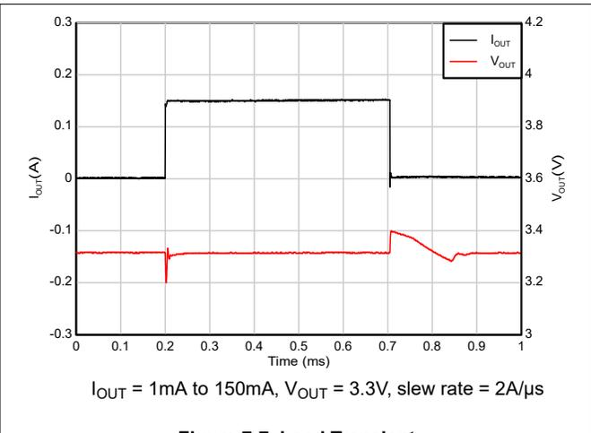
**Figure 7-7. Load Transient**
