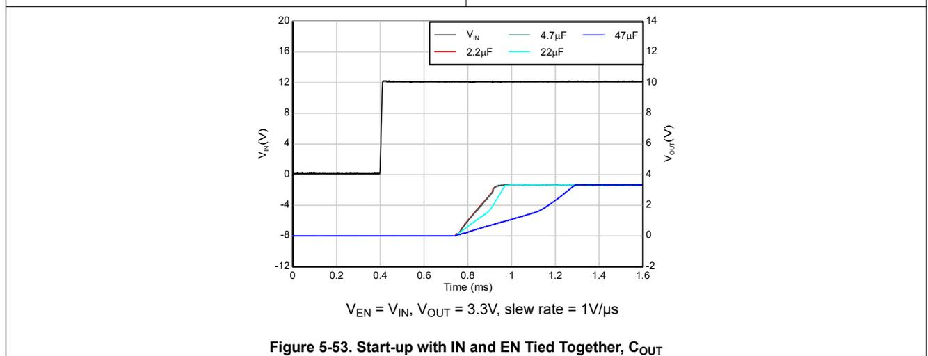
Figure 5-53. Start-up with IN and EN Tied Together,  $C_{OUT}$
