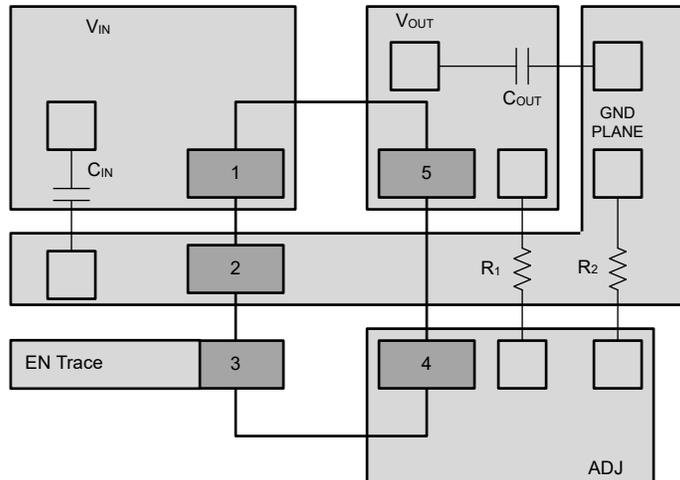
Figure 7-11. Example Layout for TPS7E81, DBV Package
