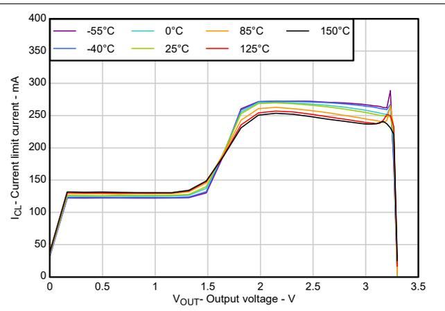
Figure 5-10. Current Limit vs Output Voltage
