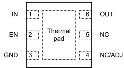
**Figure 4-2. DRV Package (Fixed/ADJ), 6-Pin WSON (Top View)**
