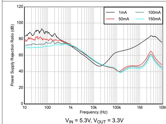
Figure 5-21. Ripple Rejection vs Frequency, Output Current
