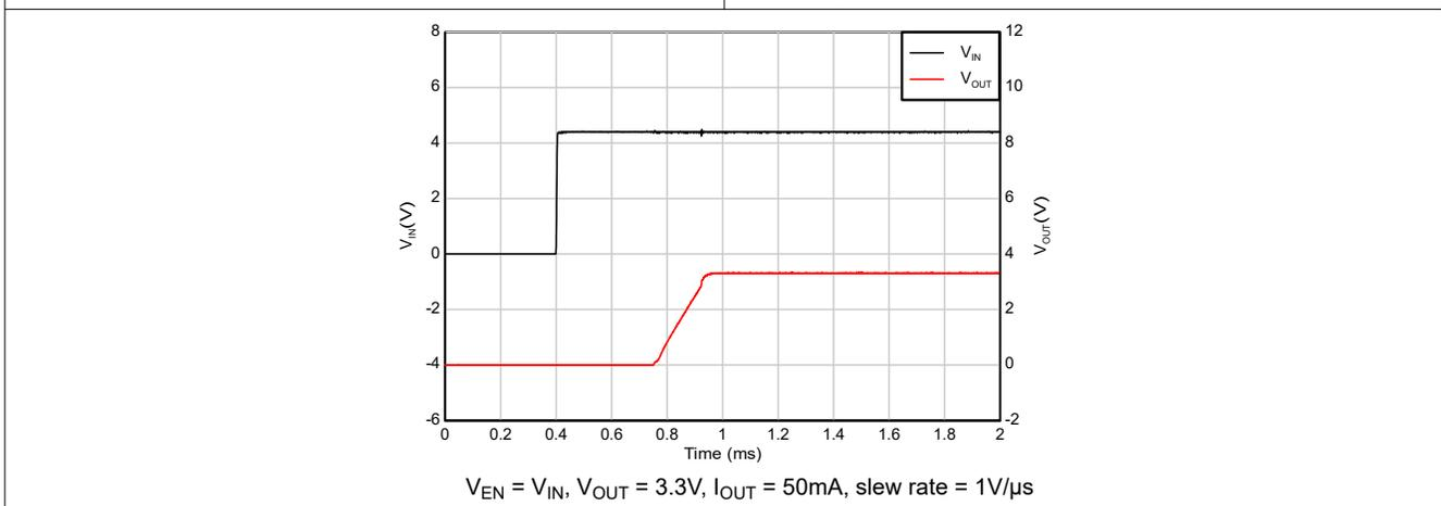
**Figure 7-10. Start-up with IN and EN Tied Together**
