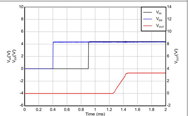
**Figure 5-48. Start-up with Sequencing (IN after EN)**
