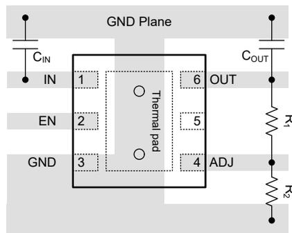
Figure 7-12. Example Layout for TPS7E81, DRV Package
