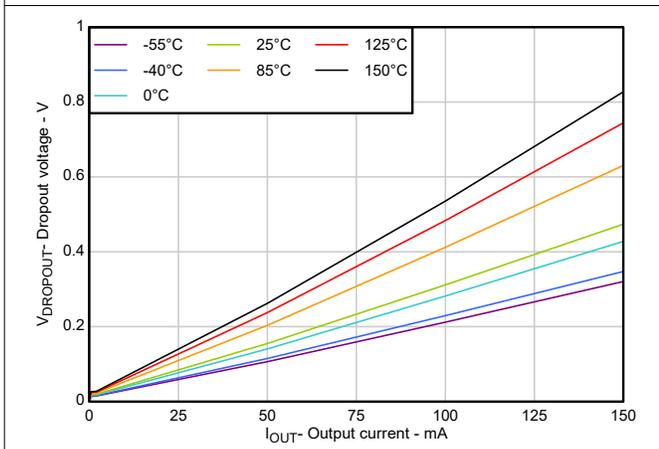
Figure 5-9. Dropout vs Output Current
