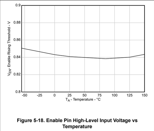
Figure 5-18. Enable Pin High-Level Input Voltage vs Temperature
