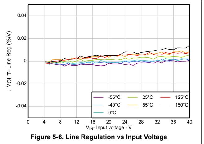
Figure 5-6. Line Regulation vs Input Voltage
