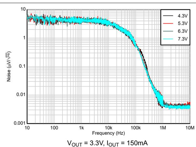
Figure 5-24. Output Noise vs Frequency, Input Voltage
