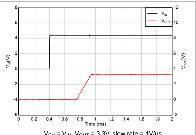
Figure 5-50. Start-up with IN and EN Tied Together
