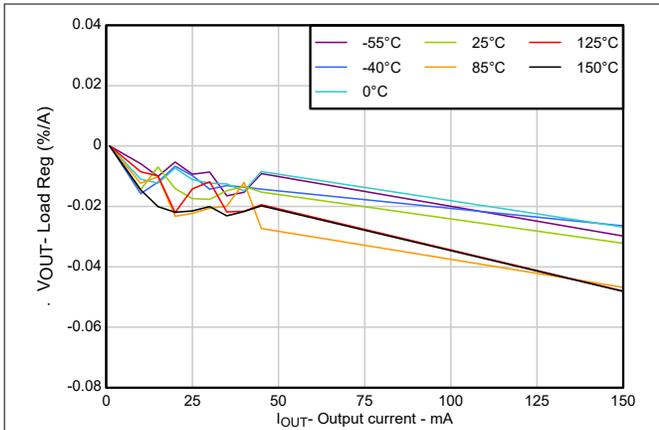
Figure 5-7. Load Regulation vs Output Current
