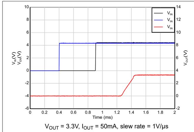
Figure 5-49. Start-up with Sequencing (IN after EN)
