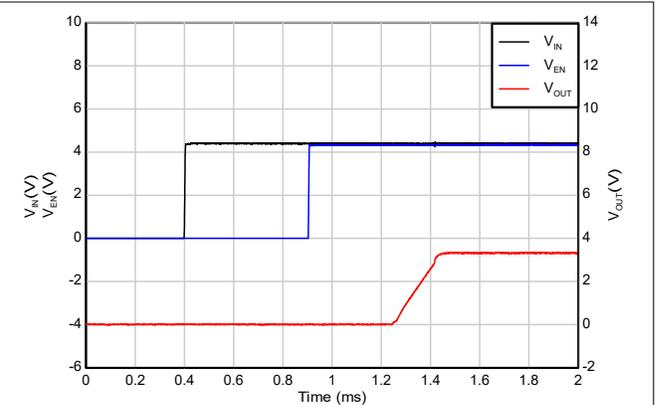
**Figure 5-44. Start-up with Sequencing (EN after IN)**
