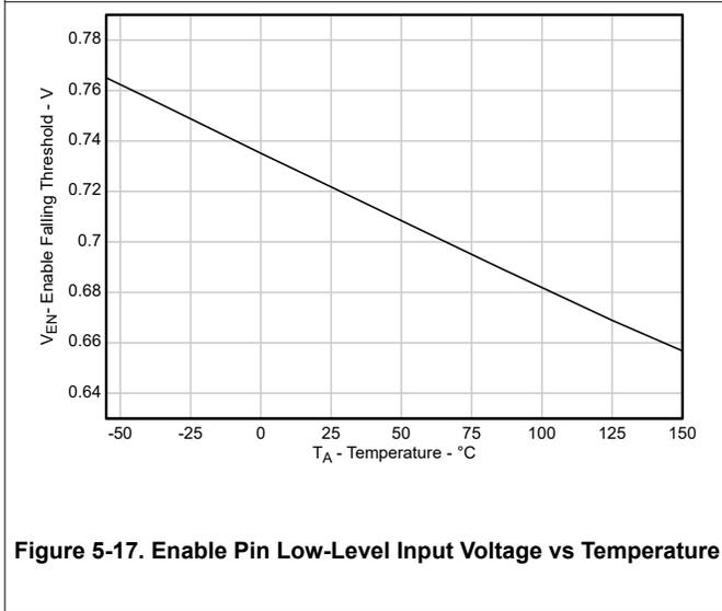
Figure 5-17. Enable Pin Low-Level Input Voltage vs Temperature
