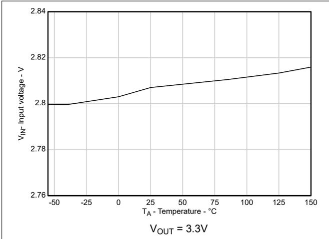
Figure 5-1. Rising Input Supply UVLO vs Temperature
