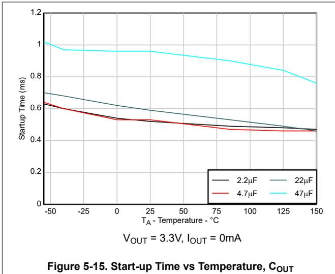
Figure 5-15. Start-up Time vs Temperature,  $C_{OUT}$
