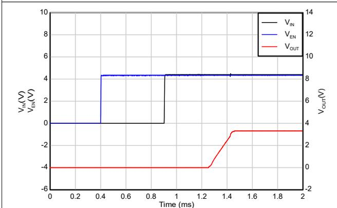
**Figure 5-47. Start-up with Sequencing (IN after EN)**
