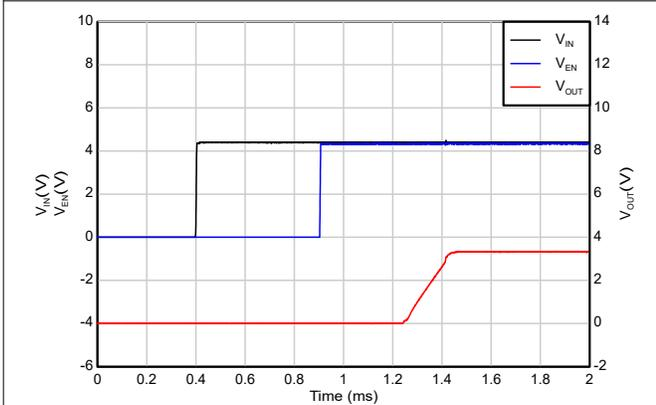
**Figure 5-45. Start-up with Sequencing (EN after IN)**
