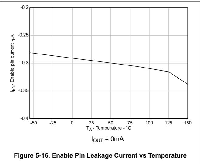
Figure 5-16. Enable Pin Leakage Current vs Temperature
