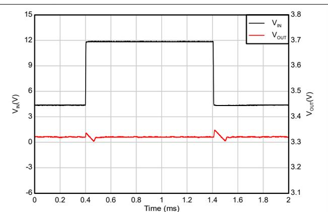
**Figure 7-12. Line Transient (4.3V to 12V)**
