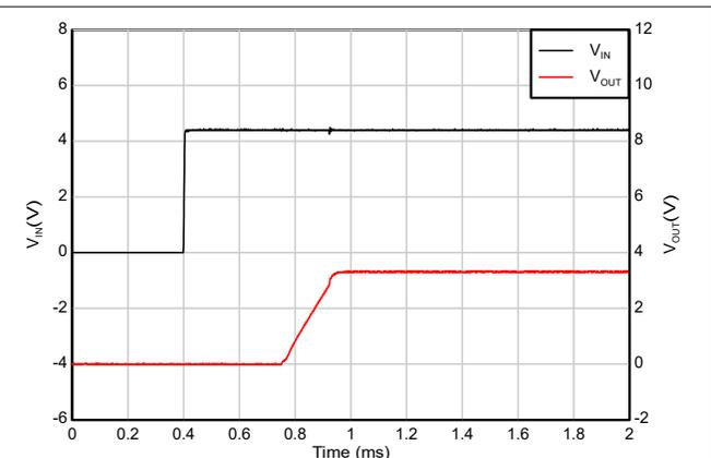
**Figure 7-10. Start-up with EN &  $V_{IN}$  tied together**
