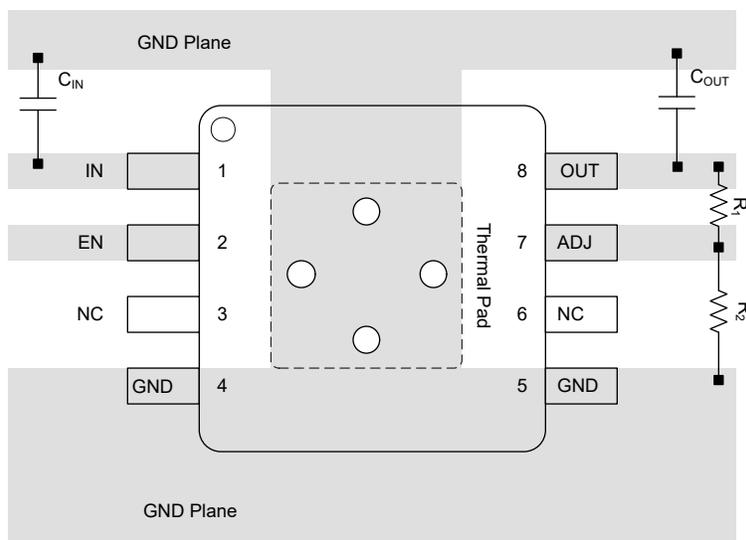
**Figure 7-19. Example Layout for the DGN Package**
