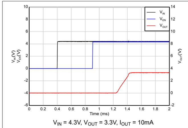
**Figure 5-33. Start-up with sequencing (EN after  $V_{IN}$ )**
