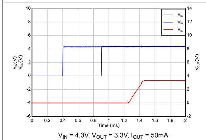
**Figure 5-37. Start-up with sequencing ( $V_{IN}$  after EN)**
