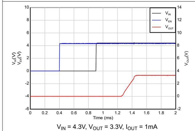
**Figure 5-35. Start-up with sequencing ( $V_{IN}$  after EN)**
