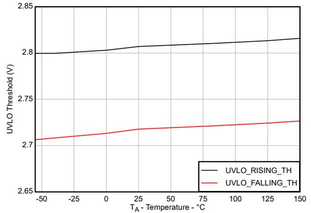
Figure 5-14. UVLO Threshold ( $V_{UVLO+}/V_{UVLO-}$ ) vs Temperature
