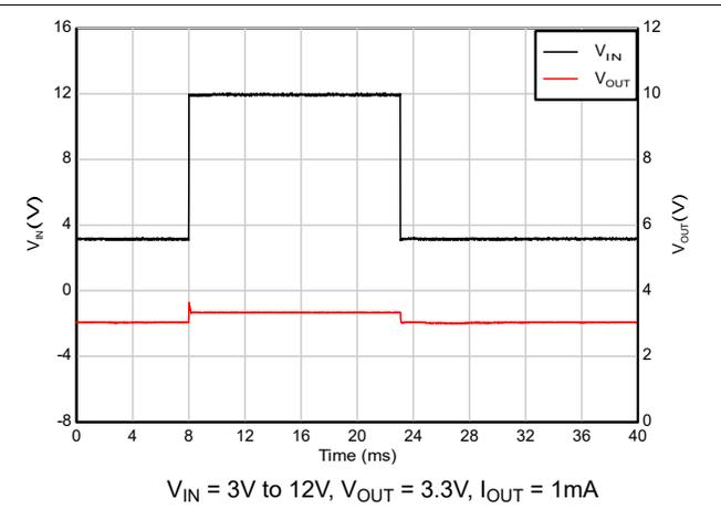
Figure 5-48. Cold-crank Recovery
