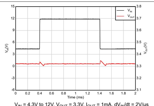
**Figure 5-38. Line Transient (4.3V to 12V)**
