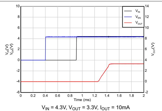
**Figure 5-36. Start-up with sequencing ( $V_{IN}$  after EN)**
