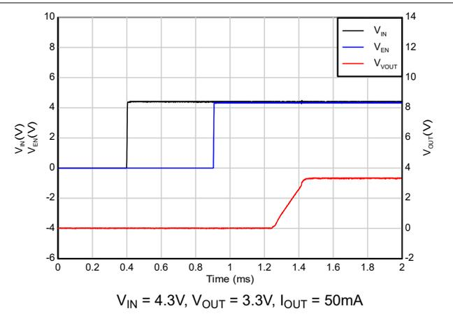
**Figure 5-34. Start-up with sequencing (EN after  $V_{IN}$ )**
