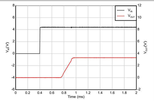
**Figure 7-8. Start-up with EN &  $V_{IN}$  tied together**
