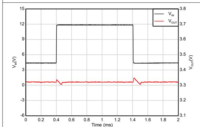
**Figure 7-11. Line Transient (4.3V to 12V)**
