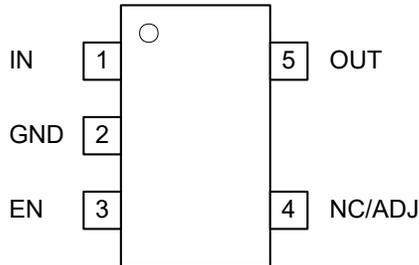
Figure 4-3. DBV Package, (Fixed/ADJ), 5-Pin SOT-23 (Top View)
