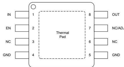
Figure 4-5. DGN Package (Fixed/ADJ), 8-Pin HVSSOP (Top View)
