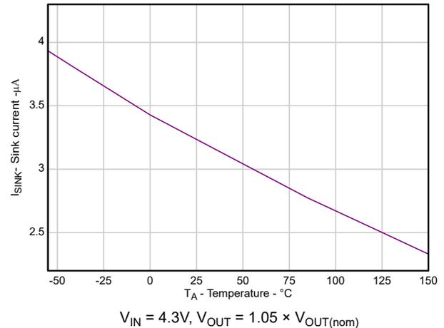
Figure 5-16. Sink Current on Output ( $I_{SINK}$ ) vs Temperature
