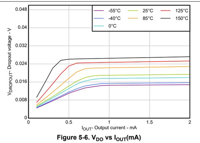
Figure 5-6.  $V_{DO}$  vs  $I_{OUT}(\text{mA})$
