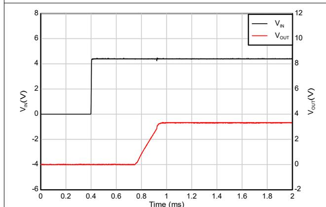
**Figure 7-9. Start-up with EN &  $V_{IN}$  tied together**
