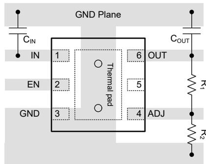
**Figure 7-22. Example Layout for the DRV Package**
