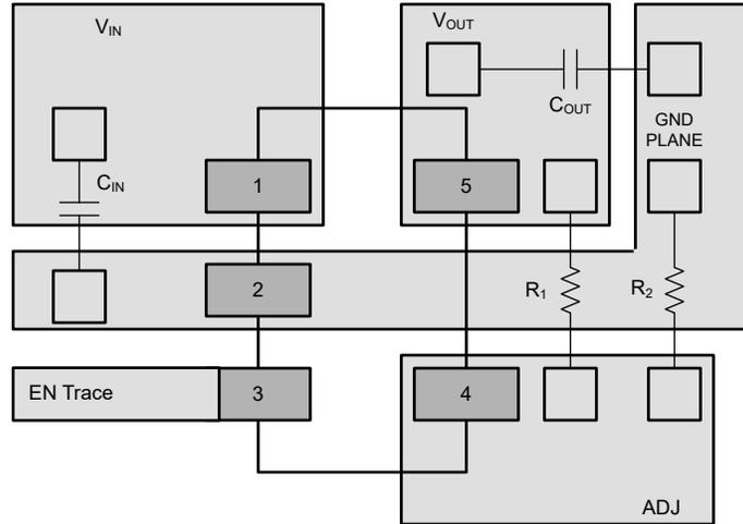
**Figure 7-20. Example Layout for the DBV Package**
