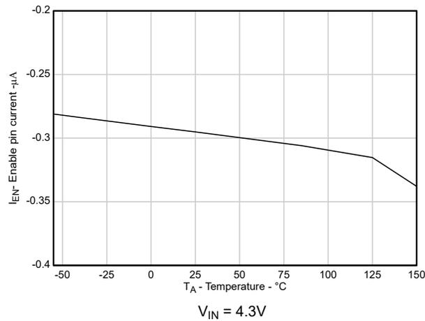
Figure 5-15. EN Leakage Current  $I_{EN}$  vs Temperature
