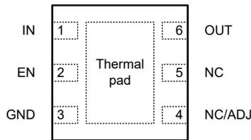
Figure 4-1. DRV Package (Fixed/ADJ), 6-Pin WSON (Top View)
