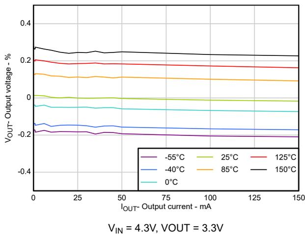
Figure 2-1. V<sub>OUT</sub> Accuracy vs I<sub>OUT</sub>
