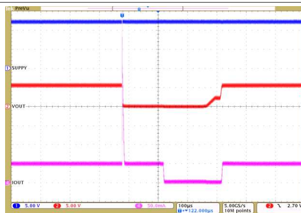
Figure 11. LED Short-Circuit Protection and Recovery
