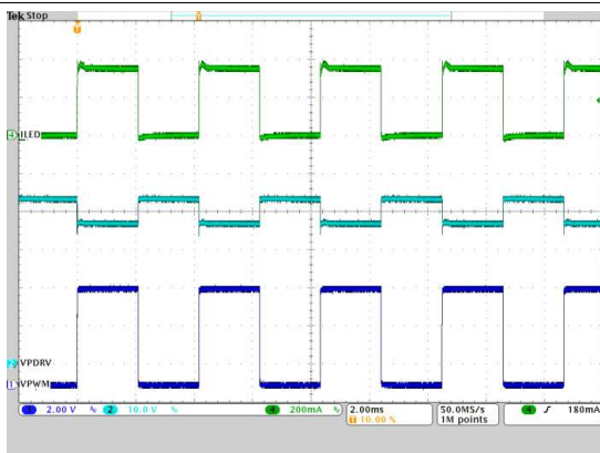
Ch1: External PWM input signal; Ch2: PDRV voltage; Ch4: LED current; Time: 2 ms/div
