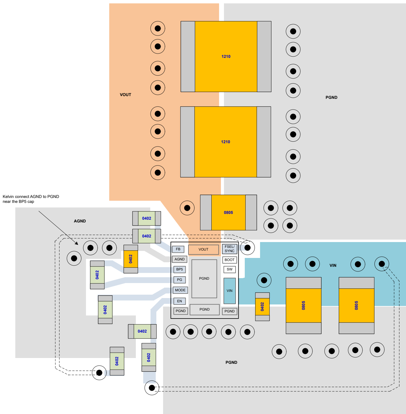
Figure 7-19. Example PCB Layout
