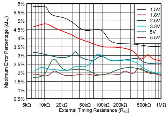
Figure 5-25. Maximum Output Pulse Width Error (Absolute Value) Versus Timing Resistor Values
