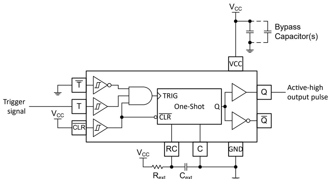
Figure 8-1. Pulse Generator Schematic Using the TPUL2G122x
