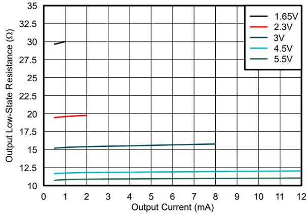
**Figure 5-4. Output Low-State Resistance vs Output Current**
