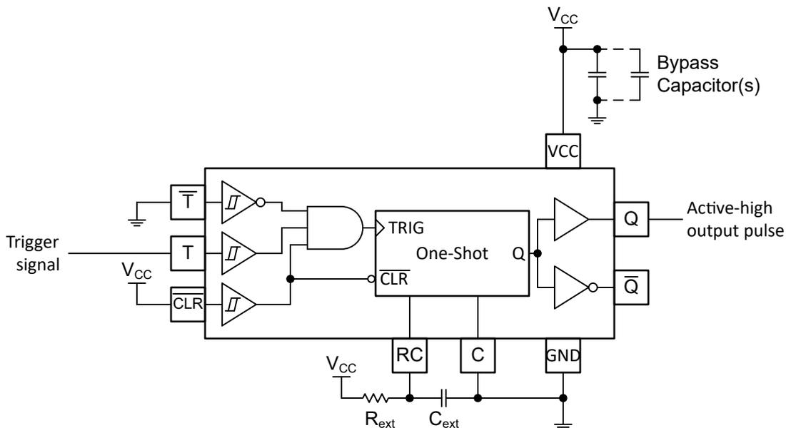
Figure 8-1. Pulse Generator Schematic Using the TPUL2G123-Q1
