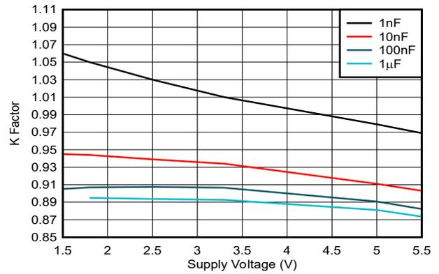
**Figure 5-7. K Factor vs Supply Voltage,  $R_{ext} = 10k\Omega$**
