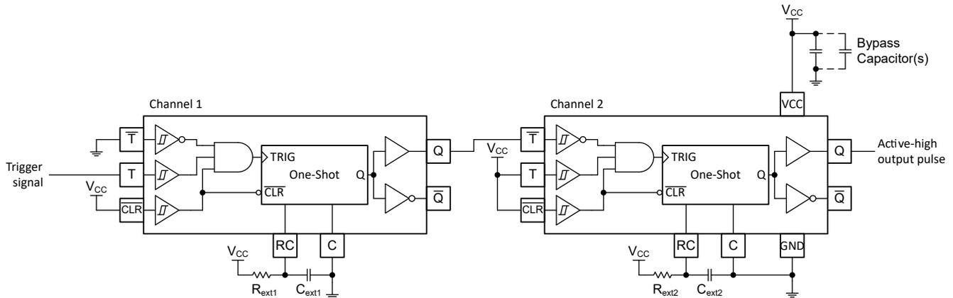
Figure 8-4. Delayed Pulse Generation Schematic Using the TPUL2G123-Q1
