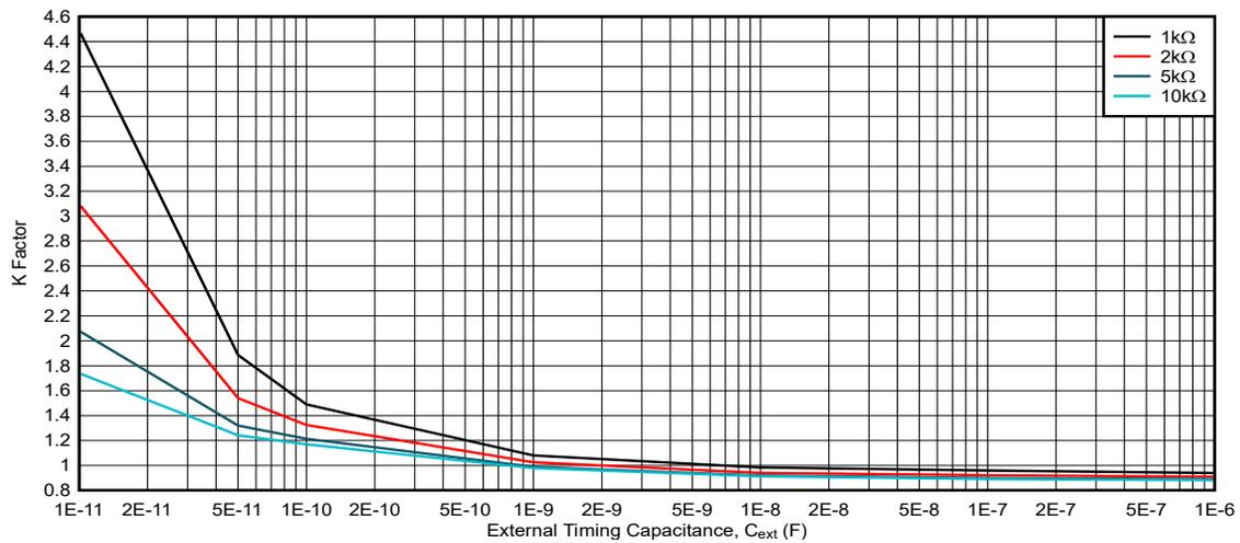
**Figure 5-16. K Factor,  $V_{CC} = 5V$ ,  $R_{ext} = 1k\Omega$  to  $10k\Omega$**
